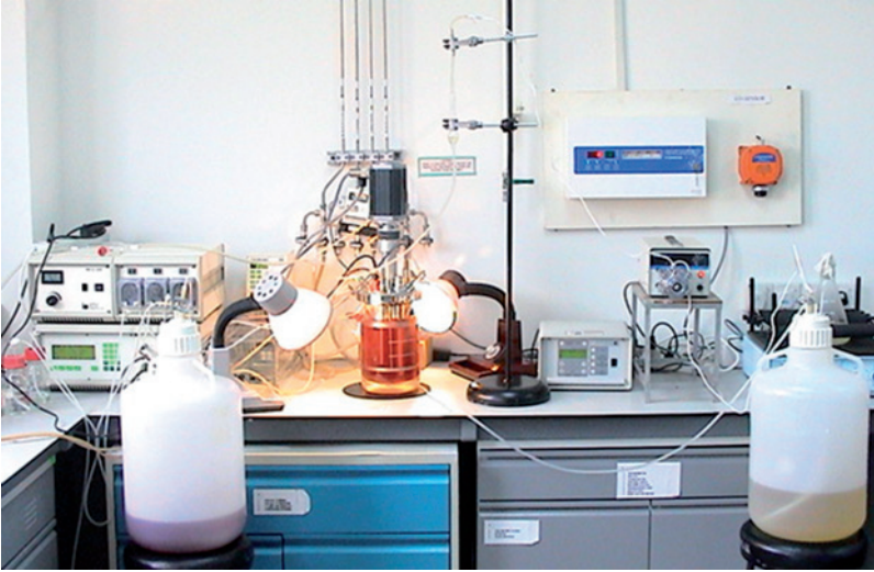
FIG. 10.7. A complete laboratory set-up of biostat, B. Braun fermenter with external feed pumps and product reservoirs.
