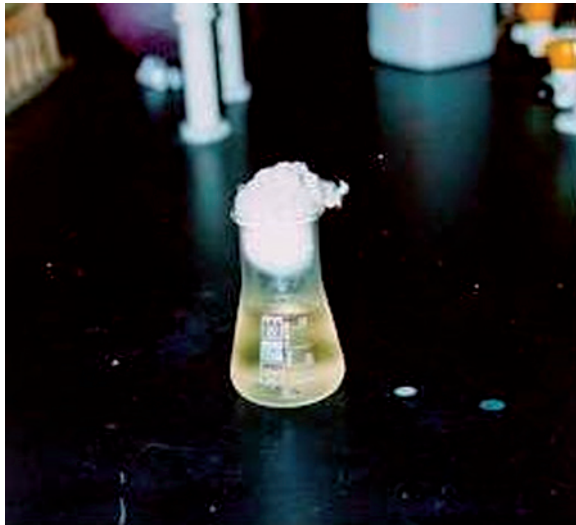
FIG. 10.3. A 50 ml seed culture is used for inoculation of batch fermenter.
