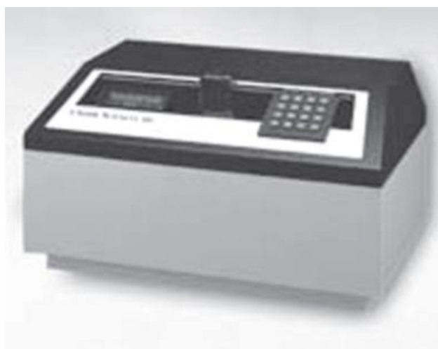
Figure 5.5 The Charm II detection system for receptor-based radioimmunoassays. (Schematic diagram provided courtesy of Charm Sciences Inc.)
