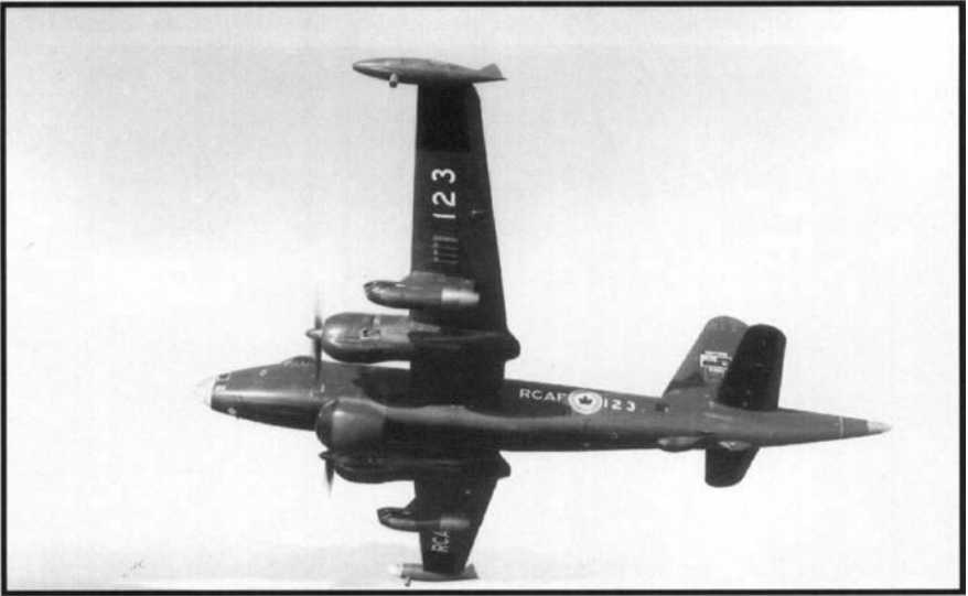
RCAF Maritime Air Command Neptune #24123 from Station Comox, equipped with jet pods and tip tanks, 29 April 1960. The Mk 101, and later the Mk 57, could be carried inside the bomb bay. DND negative PCN-1825.
