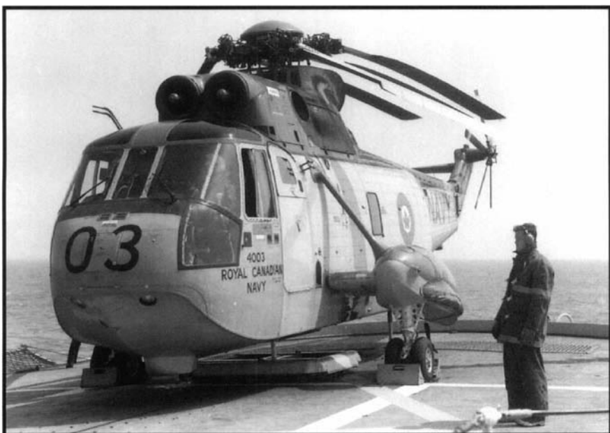
RCN CHH-2 Sea King on HMCS Assiniboine, DDE-234, 04 August 1964. A single Mk 101 or Mk 57 could be carried on the outboard starboard store.
