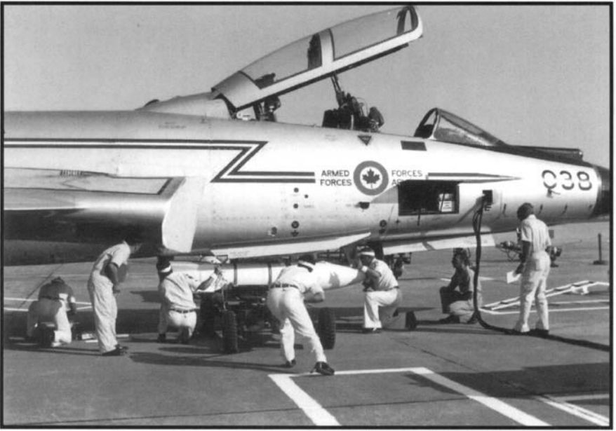
Genie rocket being positioned under CF-101B VooDoo CAF-038 by ground crew. 1977. DND negative BNC77-2841, Wallet #463, Neg. frame #23A.
