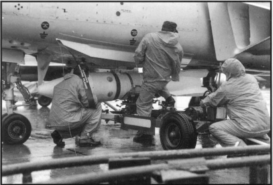
Genie rocket being uploaded rotary bomb-bay door of a CF-101B at the "William Tell 1976" air weapons competition at Tyndall AFB, Florida, on 7 December 1976. DND negative NBC76-1940 Wallet #457, Neg. frame #18A.
