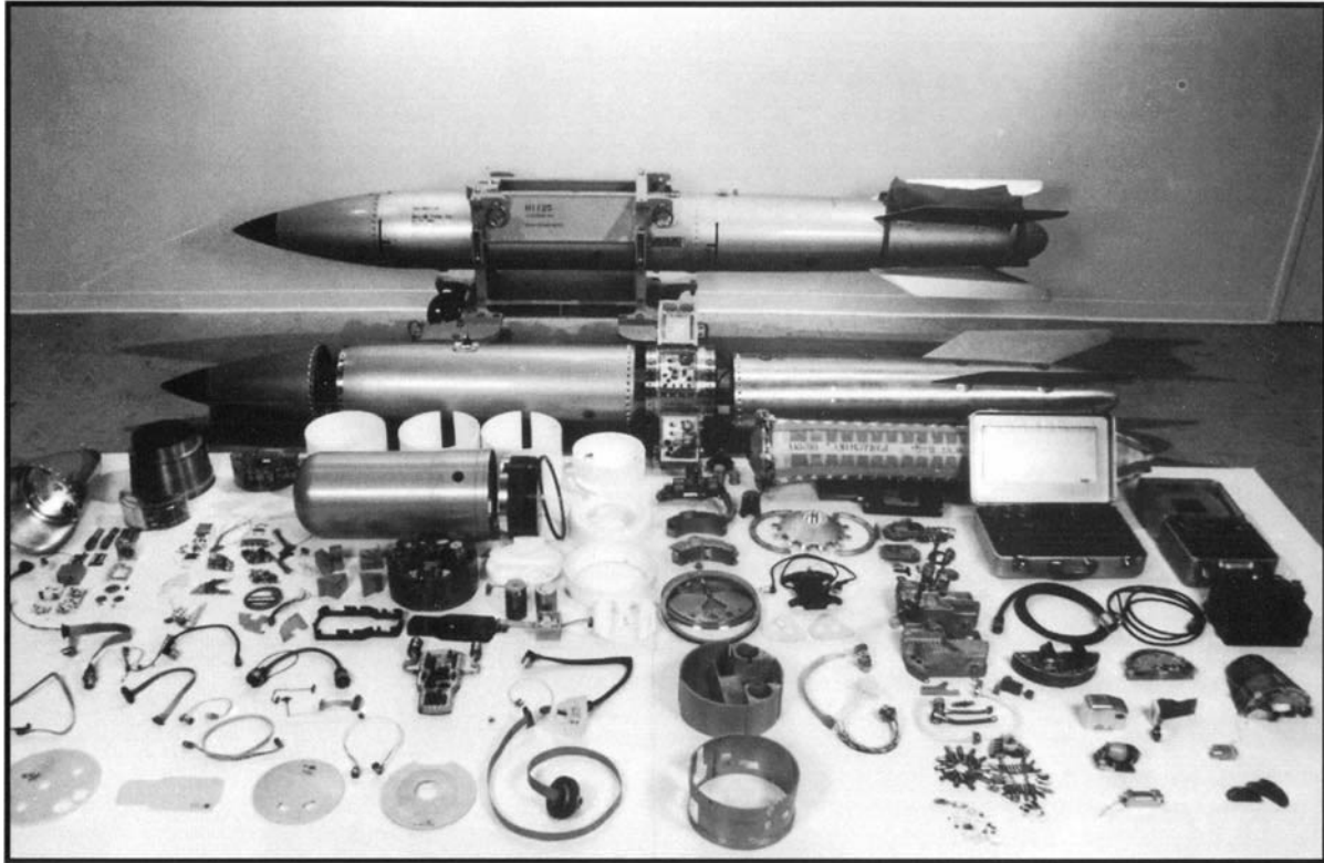
Although not used by Canada, the B-61 was a contemporary of and replacement for the Mk 28 and Mk 43 bombs. This shows some of the more than 6000 parts in this 3.6-metre-long thermonuclear gravity bomb.
