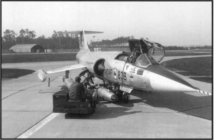
Four man crew load a Mk 28RE on the centre pylon of CF-104 #12838 at 4 Wing, Baden-Soellingen, inside a double-fenced compound using an MJ-1 bomblifter truck. DND negative PCN 69-109.
