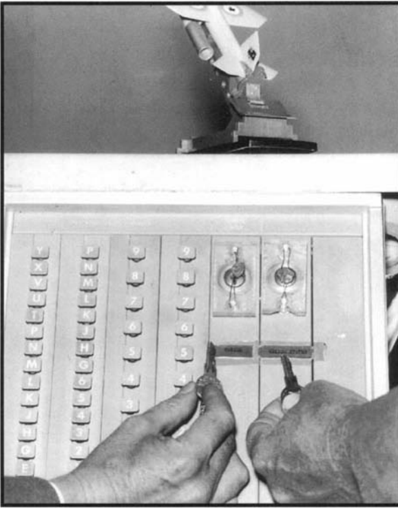
Part of the BOMARC control panel showing the two-key concept (Dual Key) with both Canadian and US keys, and sealed key-holes covered with special sealing wax and wires. Station North Bay, May 1965. DND negative PCN 5528.
