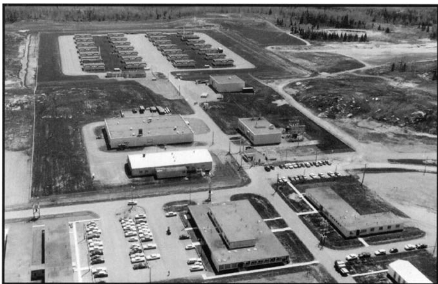
Aerial photograph of the Station La Macaza BOMARC site showing 28 missile shelters, 2 erect BOMARCs in shelters #11 (top centre), and #18 (left), security perimeter and gate, ordnance building/SAS, and composite building.
