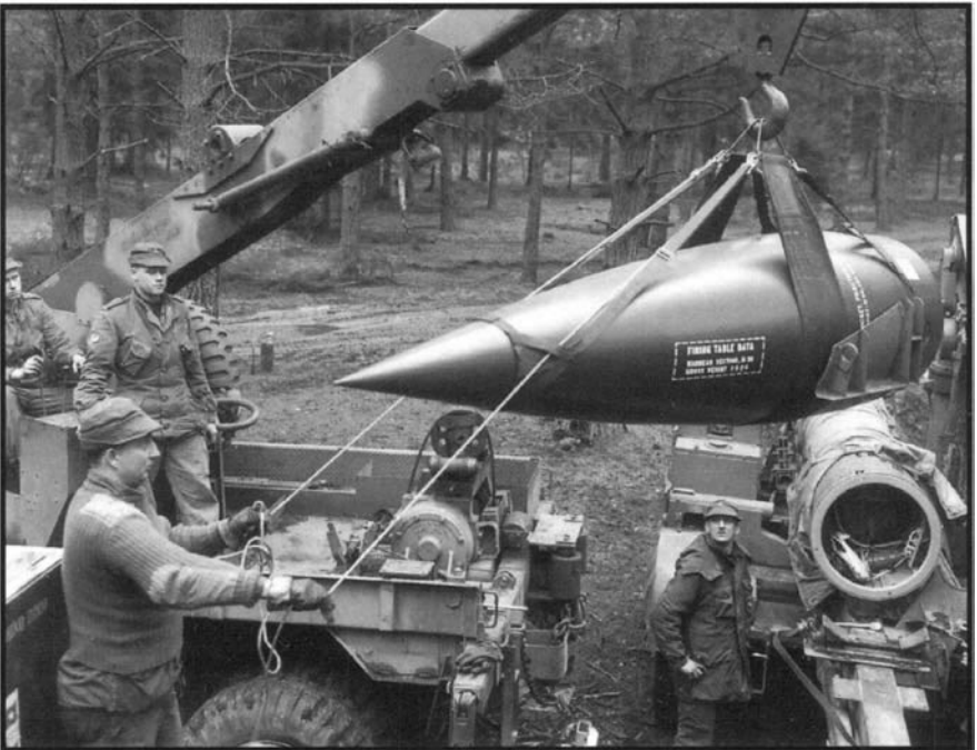
Honest John training warhead is mated by crane to an Honest John rocket of the 1 SSM Battery at 1 RCHA Gun Camp, Munsterlager, Germany, 24–25 April 1969.
