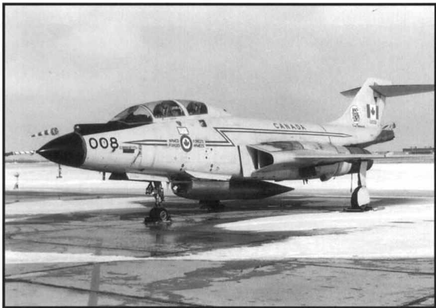
CF-101B VooDoo 101008 sits idle in Winnipeg ten years after the nuclear Genies had been removed from its base at CFB Chatham. A baggage pod has replaced the weapons. Photo by author.
