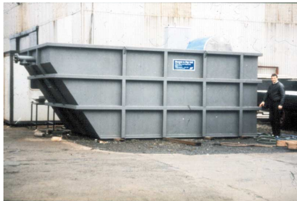
Fig. 5.56. Packaged activated sludge plant for a population of 500 with a small horizontal rotor aerator ready to be taken to site for installation.
