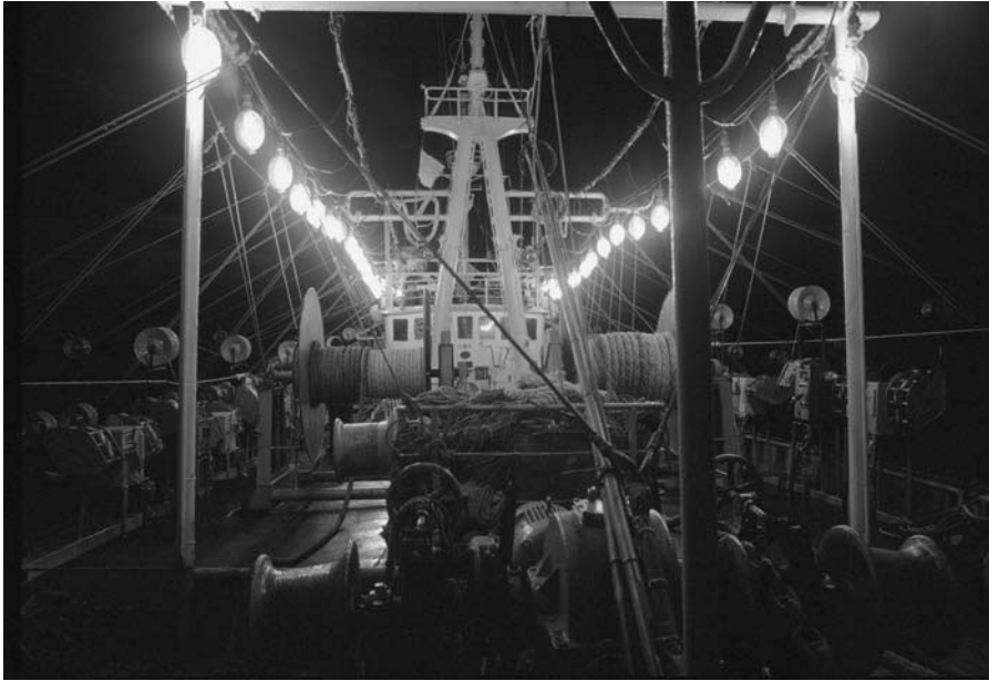
Fig. 18.2 Deck of a Japanese squid-jigging vessel at night showing the rows of incandescent fishing lights and fishing gear in place.
