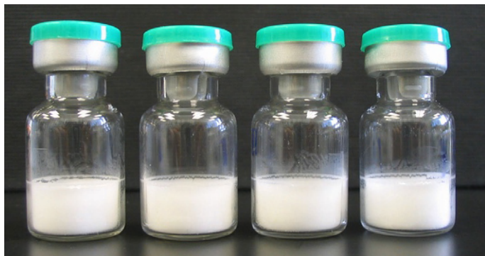
Figure 18.2 Freeze-dried cakes of camptothecin nanomedicines (CPT-SSM) at an initial concentration of 15 mM DSPE-PEG 2000 and CPT:DSPE-PEG 2000 molar ratio = 0.004:1. N = 4 , of 1 ml filled vials placed in different positions on the tray, and subjected to a controlled lyophilization cycle by the Virtis Genesis 25 EL freeze dryer, including slow freezing of the samples by decreasing the temperature at 0.25 °C/min to -40 °C. In the first step of the freeze-drying process, the shelf temperature was maintained at 0 °C for 3.5 h, followed by an additional drying step of 7 h at 0 °C under a pressure of -55 \times 10^{-3} mmHg. The condenser temperature ranged from -77.5 °C to -83.6 °C.
