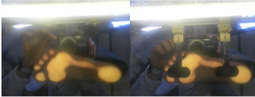
Fig. 22. Pictures of feet sole reflected by the podoscope mirror, a) without electrodes, b) with 27 cm 2 electrodes
