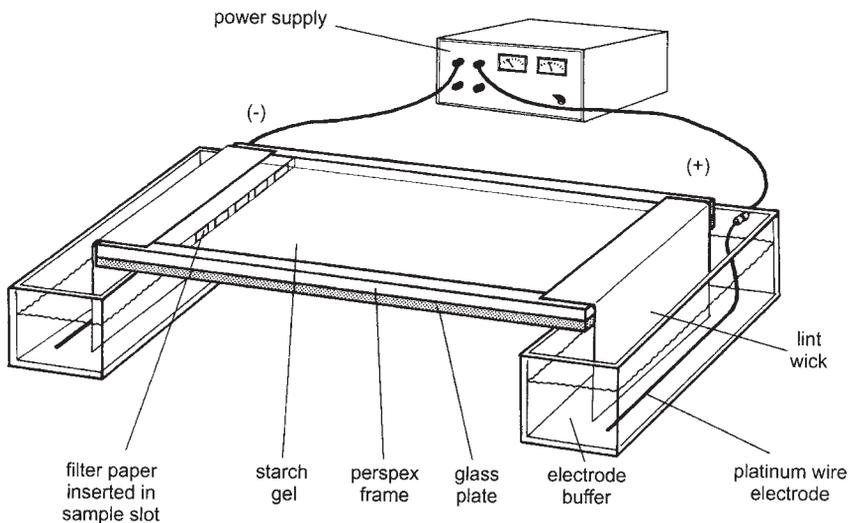
**Fig. B2.3a** Apparatus for the separation of allozymes by horizontal starch gel electrophoresis (courtesy Chris Beveridge).
