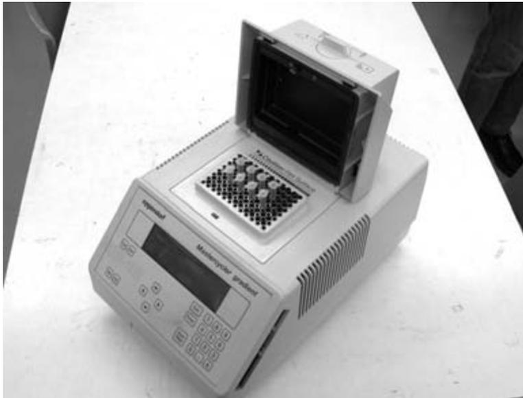
**Fig. B2.2a** A thermal cycler in which PCR is carried out. During PCR the heated lid is closed over the microtubes which are positioned in the heating block.
