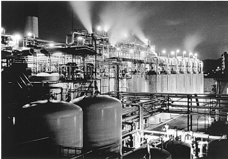
Figure 14.10 Amino acid production plant of Kyowa Hakko in Japan showing on the right seven large fermenters each 240 m 3 in size, suitable for L-glutamate production.
