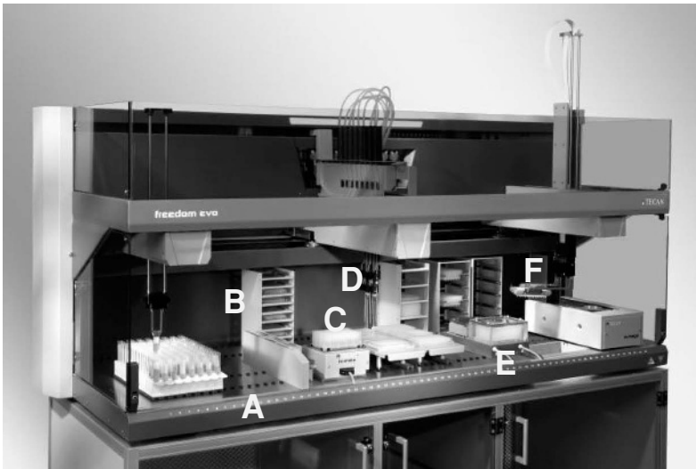
Figure 12.4 Photograph of a commercial robotic platform for performing high-throughput cell screening and optimisation experiments in microtitre plates. The items on the robotic deck (A) are mapped in the controlling software. The cultivation itself is performed on a heated plate shaker (C) and growth media, or culture broth, are dispensed using the liquid handling pipettes (D) into secondary microtitre plates housed in the hotel (B). Some preliminary cell harvesting stages can also be performed in microtitre plates and centrifuges and filtration devices (E) can be incorporated onto the platform. The microtitre plate grabber (F) is used to move plates around the deck and between the various unit operations and analytical devices. In this way it is possible to perform the entire cultivation process without human intervention whilst data collection is fully automated (image courtesy of Tecan UK Ltd).
