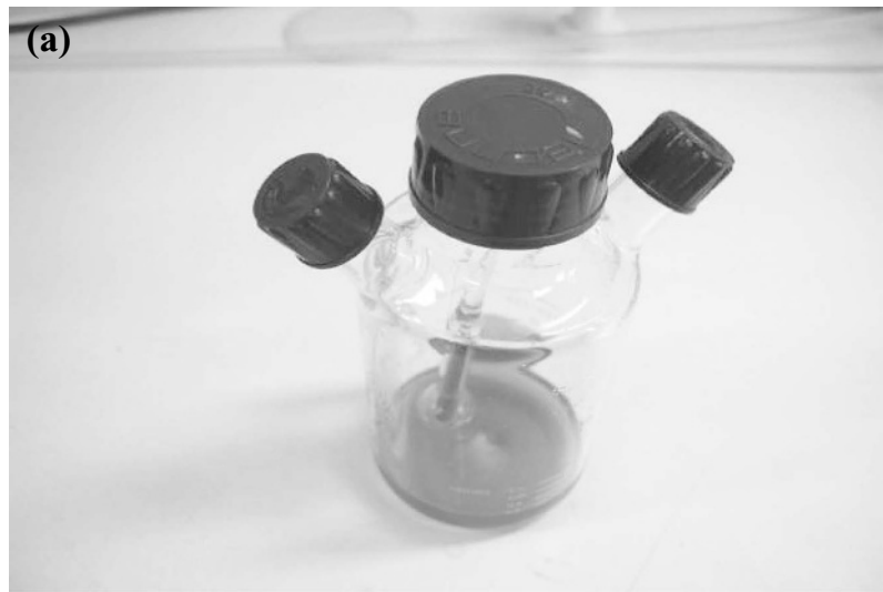
Figure 22.8 Spinner flask (a) and 5-l laboratory-scale bioreactor (b) routinely used for both insect and mammalian cell culture.
