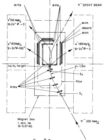
Fig. 10. Layout for  $\pi^{\circ} \rightarrow e^{+}e^{-}$  in the Omicron spectrometer.
