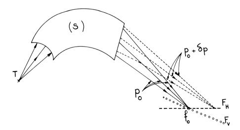
Fig. 2- Focal surfaces of the Spectrometer.
