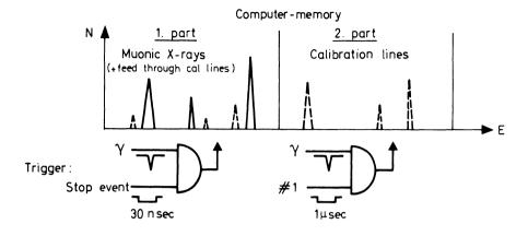
Method I : External  $\gamma$ -source triggered with beam particles
