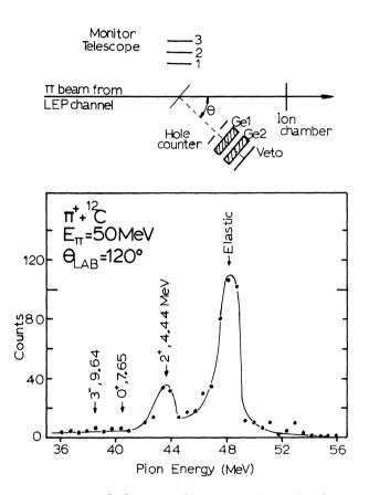
Fig. 1. Upper portion of figure shows a schematic diagram of the experimental set-up (see text). Lower portion shows pion scattering spectrum for 50 MeV  $\pi$  at a lab. angle of 120°. Note the clean separation of the elastic peak from the first inelastic state (2<sup>+</sup>, 4.44 MeV). Spectrum includes only pions stopping in the second Ge crystal.
