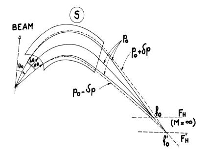
Fig. 3- Kinematical displacement of the horizontal focal surface.
