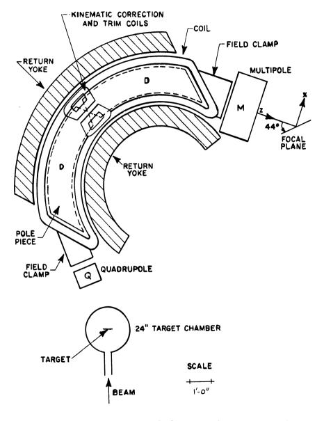
Fig. 4. Layout drawing of the magnetic spectrograph
