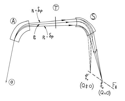
Fig. 4- Compensation of the primary beam energy dispersion.
