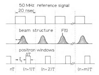
Fig. 7. Schematic arrangement of the reference signal the muon beam bursts and the time windows of observation for the strobo-scopic method.
