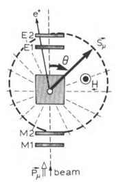
Fig. 4. Schematic experimental arrangement in a transverse field. The asymmetric decay pattern is rotating past the counters.
