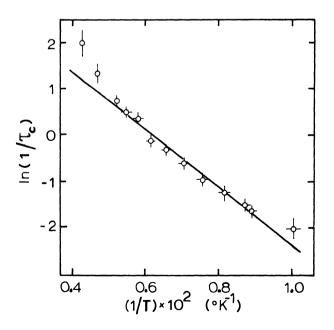
Fig. 17b. Dependence  $\ln(1/\tau_c) = f(1/\tau)$  obtained from the relaxation rates in Cu.
