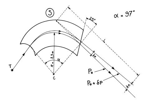
Fig. 1- Schematic view of the Spectrometer and it's Dispersive properties.
