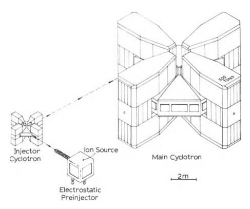
Fig. 1. Approximate scale drawing of the three-stage accelerator
