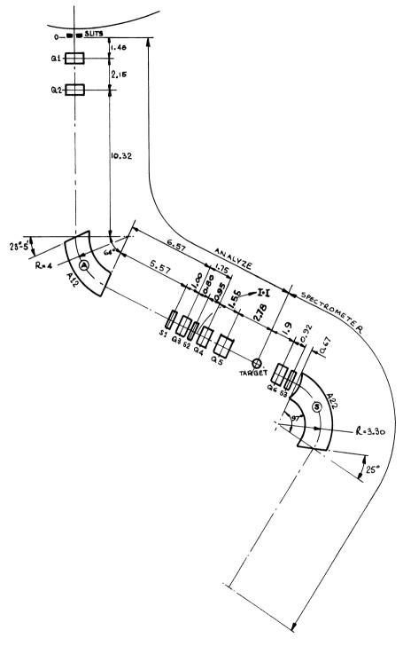
Fig. 6- Layout of the whole Spectrometric Line.
