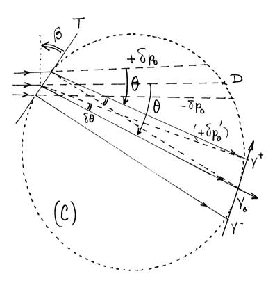
Suppose that the incident beam is dispersed as indicated on the figure as a function of the momentum difference ( $\pm \delta p_0$ ) compared to the central value  $p_0$ . Then for an incident particle having a momentum ( $p_0 + \delta p_0$ ), the scattered particle at the physical angle  $\theta$  will have a momentum ( $p'_0 + \delta p'_0$ ), the ratio  $\delta p'_0 / \delta p_0$  being fixed by the kinematics of the reaction.
