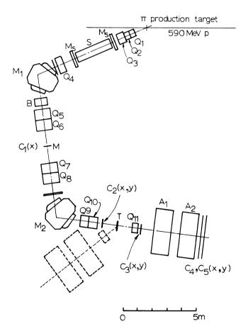
Fig. 1. Layout of High Resolution  $\pi$ -channel
