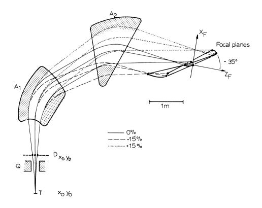
Fig. 2 . Layout of  $\pi$ -Spectrometer
