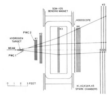
Fig. 2. Plan view drawing of the Argonne Effective Mass Spectrometer, including proportional wire chambers added for experiment E-336. Recoil counters used in the elastic scattering trigger are not shown.
