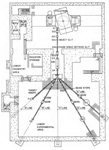
FLOOR PLAN CYCLOTRON CAVE-LOWER EXPERIMENTAL AREA
