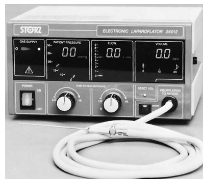
FIGURE 3-16 Gas insufflation unit for laparoscopy. Gauges that measure gas supply, intra-abdominal pressure, gas flow rate, and amount of gas insufflated are located on the front of the unit. A Veress needle is shown connected to the gas insufflation tubing by a Luer-Lok attachment.
