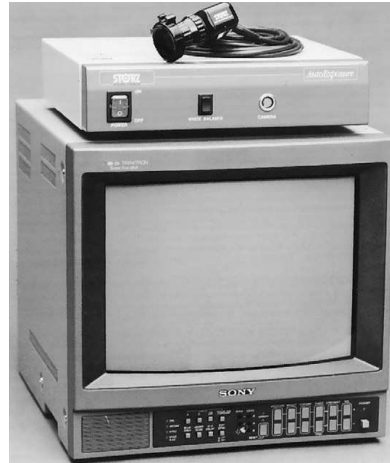
FIGURE 3-2 High-resolution endoscopic video camera and monitor. The camera (top) is attached to the eyepiece of the endoscope. The endoscopist performs the procedure while watching the image on the video monitor. The camera can be fully immersed and features automatic exposure control.
