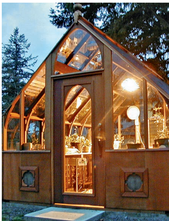
Ordinary incandescent lights aren't particularly good sources of growth-promoting light, but they can help heat a greenhouse. And their attractive warm light also turns a greenhouse into a nighttime landscape design feature.
