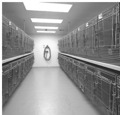
Figure 9.2 Hanging cage rack system for mature macaques. Pair housing is accomplished through commingling doors on the side of adjacent cages.
