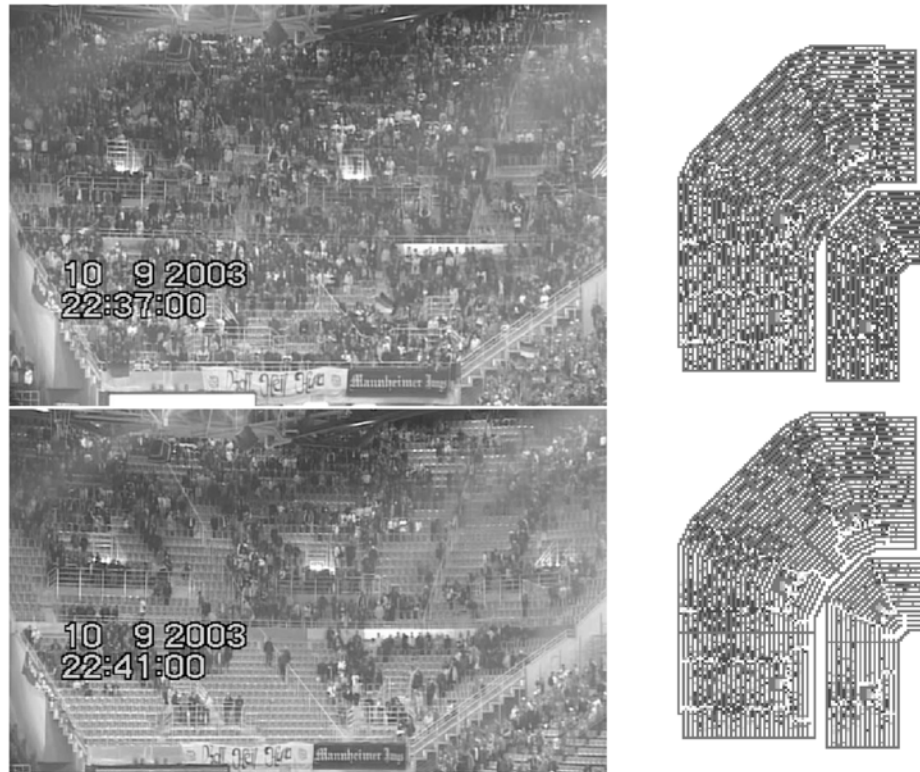
Figure 13. Comparison of the results for the video analysis (left column) and the simulation (right column) at the beginning of the egress. The video snapshots are taken at (from top to bottom) t = 2 and t = 6 minutes for the videos and t = 20 seconds and t = 3 minutes for the simulation.
