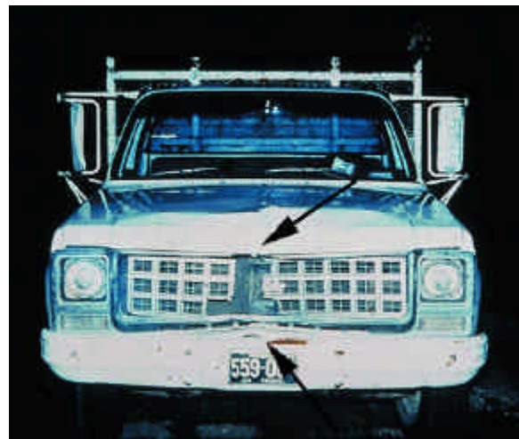
FIGURE 13.81 There were signs where the bike was struck by the front of the truck. See next photo.
