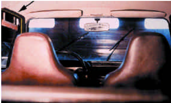
FIGURE 13.71 The car came to rest in the adjacent field and the driver was dead in the front seat. The arrow points to a ruler which is measuring the size of the open window. The driver's hat was discovered next to a fence at the point of initial impact. See next photo.
