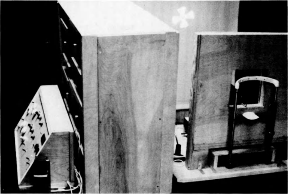
Fig. 1. The testing apparatus with stimulus presented on the screen, master control panel on the left, subject is seated with chin in chinrest.
