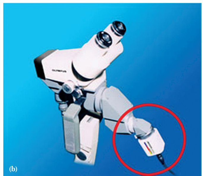
Fig. 7.5: (a) A small, light-weight three chip CCD camera. (b) A CCD camera attached to colposcope.
