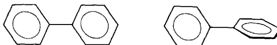
Figure 9-57. The molecular structure of biphenyl is coplanar in the crystal [9-57] while its two benzene rings are rotated by about 45^\circ relative to each other in the vapor [9-58].
