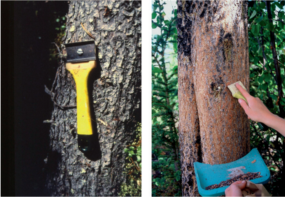
Fig. 4-4. Collection of outer bark scales from typical conifer. A paint scraper (hardened steel) of the type shown is an effective tool for this purpose.
