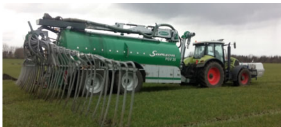
Fig. 84.1 The white box in front of the tractor contains the sulphuric acid. The acid is pumped into a tube that runs underneath the tractor and all the way down along the slurry tanker. At the rear of the wagon the acid is added to the slurry just before the slurry flows into the hoses and applied on the field. Foto: Tavs Nyord
