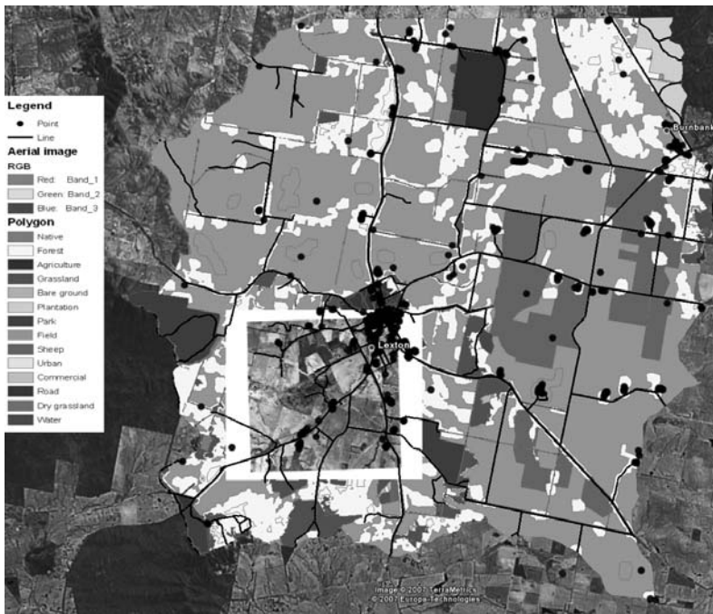
Fig. 25.4. Screen shot of Google Earth : all shapefile features and the screen overlay were imported through a KML file, the image overlay was imported with the inbuilt image module
