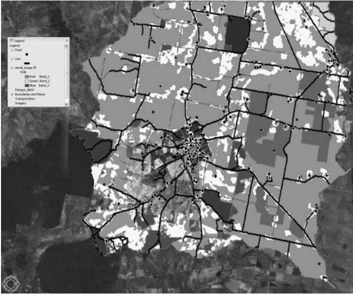
Fig. 25.2. Screen shot of ArcGIS Explorer : point, line features and imagery were imported using an inbuilt import module while the polygon feature was imported through a KML file
