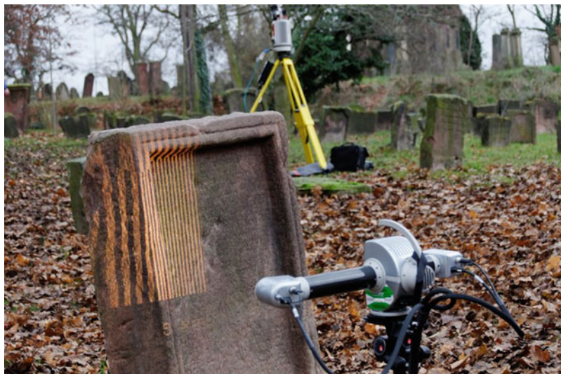
Fig. 11.9 Complementary use of two 3D sensors for capturing the Jewish cemetery Heiliger Sand near Worms, Germany. Foreground, structured light scanner Breuckmann smartSCAN 3D-HE color for scanning the headstones in micrometer accuracy; background, terrestrial laser scanner Riegl VZ-400 for scanning the entire site (image courtesy Hubert Mara)
