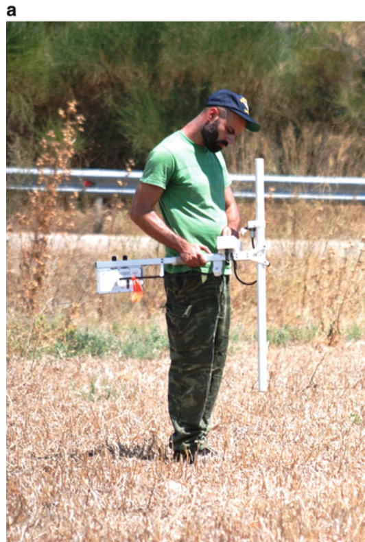
Fig. 14.10 (a) A single fluxgate gradiometer sensor of Bartington G601. (b) An eight-sensor fluxgate gradiometer array of SENSYS surveying the Neolithic tell of Perdika 2 at Central Greece. (c) Indicative results from the single sensor magnetic survey of the Agora of Sikyon in Peloponnese (Sarris et al. 2008). (d) Multisensory survey of Almyriotiki Neolithic tell at Central Greece. Results have been superimposed on a WorldView-2-satellite image (2 June 2012) (Sarris et al. 2015a)
