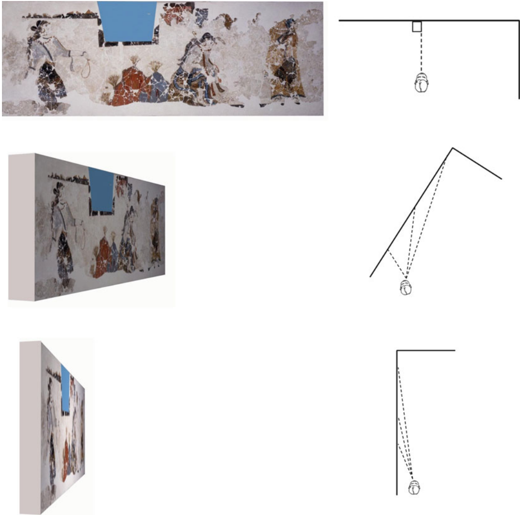
Fig. 5.7 Varying angles of incidence for a wall surface. Frontal surfaces are always easier to see
