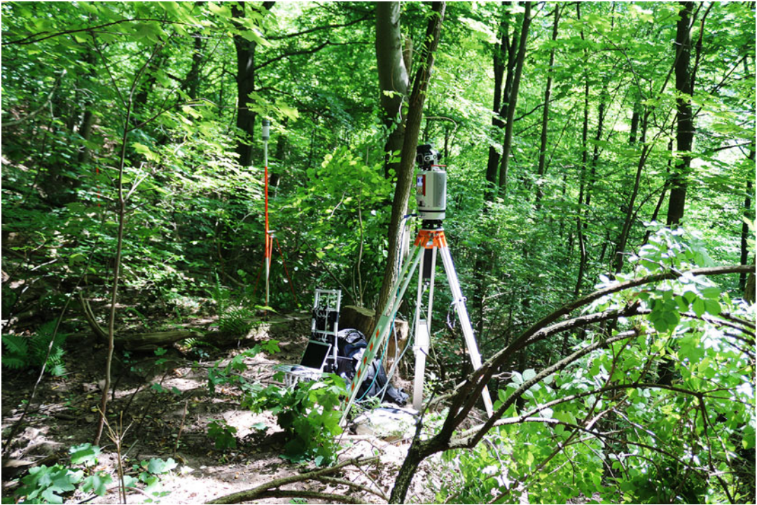
Fig. 13.2 The Riegl VZ-400 on-site with dense vegetation in the underwood
