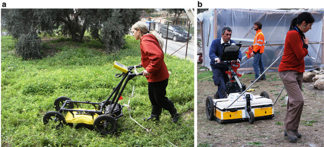
Fig. 14.2 (a) Noggin Plus (Sensors & Software Ltd.) 250 MHz GPR system in a survey at the ancient theatre of Chersonessos in Crete. (b) MALA MIRA multi-antenna GPR configuration with eight 400 MHz antenna applied in a survey at Feres (Velestino), Central Greece
