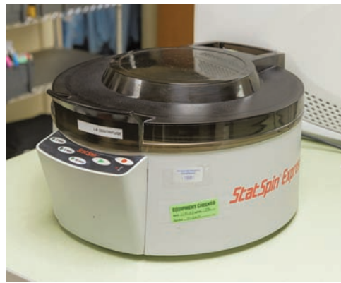
FIGURE 2-2 A centrifuge spins samples at high speeds.
