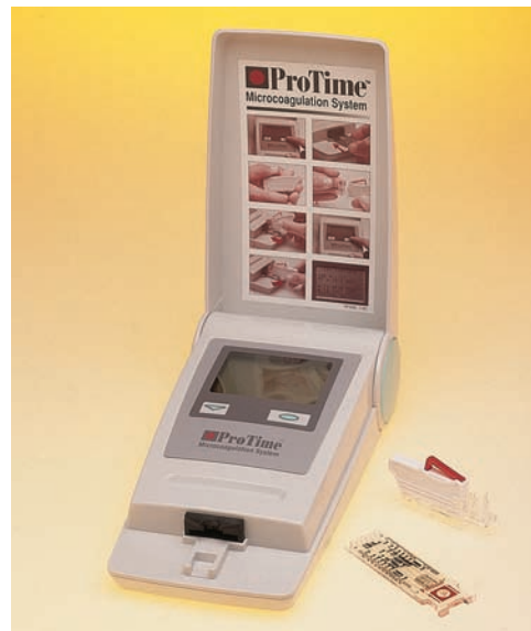
FIGURE 17-3 The ProTime Microcoagulation System for prothrombin time testing is designed to safely manage warfarin (Coumadin) therapy. (Courtesy ITC, Edison, N.J.)
