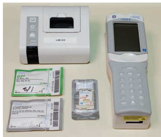
FIGURE 17-1 Handheld instruments such as the i-STAT system can perform chemistry analysis quickly and accurately. The test cards shown are for a chem 8 panel (basic metabolic panel), cTnI (troponin) and G3+ (blood gasses-pH, PCO 2 , and PO 2 ).
