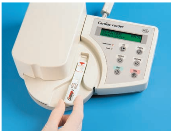
FIGURE 17-4 The Cardiac Reader system allows rapid determination of the cardiac markers troponin T and myoglobin from a single whole blood sample. (Courtesy Roche Diagnostics, Indianapolis, Ind.)
