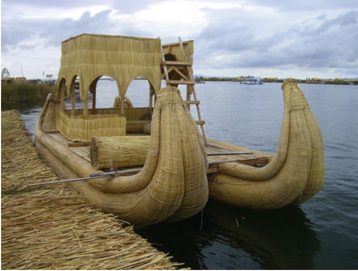
Fig. 24.6 Reed boat on Lake Titicaca, Peru. The reeds cover >2,000 two litre plastic bottles
