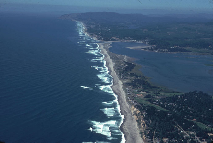
Fig. 21.3 Siletz Spit and Bay within the Lincoln City Littoral Cell on the northern Oregon coast, while to its north and south the beach is backed by high cliffs composed of coarse-grained Pleistocene marine-terrace sands (Photo P.D. Komar)
