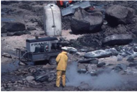
High-pressure, hot-water treatment with chemical additive to remove oil adhered to bedrock/boulder shorelines at the Tanio oil spill site, Brittany, France.
