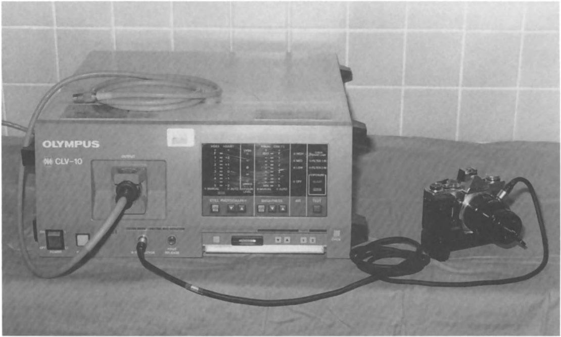
FIGURE 6.4. Olympus still photography and variable video light source, with a xenon vapor arc lamp.
