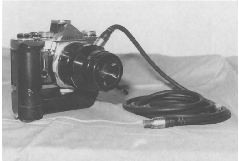
FIGURE 6.1. Close-up of the Olympus Co. endoscopic still photography system consisting of an OM-1n camera body, SM-EFR 3 combined dedicated lens/light sensor unit, and autowinder.
