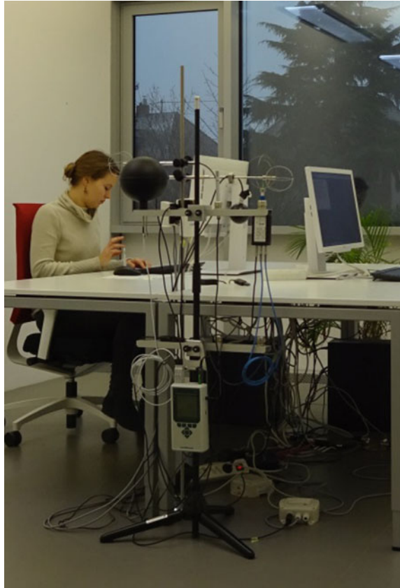
Fig. 7.17 Thermal comfort measurements at a height of 1.1 m (subjects' head level) close to the two workplaces in one of the test rooms in the LOBSTER (photo by Marcel Schweiker, KIT)
