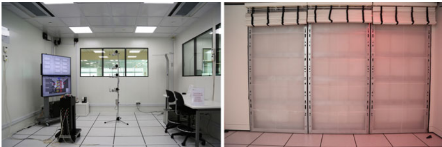
Fig. 7.5 Instrumented test room ( left ) and flexible façade system ( right ) of SinBerBEST Test Bed at BEARS (photos by BEARS)
