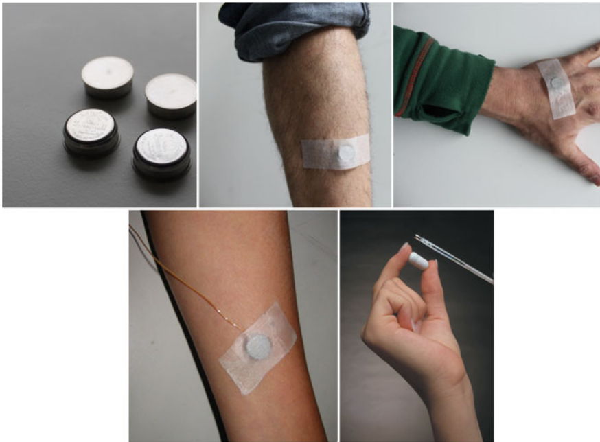
Fig. 7.19 Different sensors for temperature measurements on the body. Top iButton ® temperature sensors (photos by Michael Kleber (KIT); bottom thermocouple (left) and encapsulated CorTemp ® ingestible core body temperature sensor which can be swallowed (left photo by Hui Zhang (CBE), right photo by HQ Inc.)
