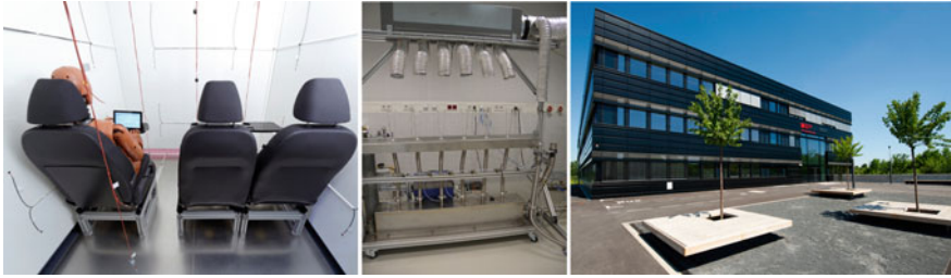
Fig. 7.7 The Comfort Cube ACCu ( left ), the set-up of the reference scale in the Indoor Air Quality lab ( middle ), and the “Living Lab” institute building at E.ON ERC ( right ) (all photos by E.ON ERC)
