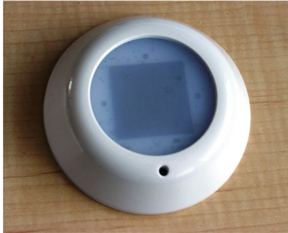
Fig. 6.4 Ceiling-mounted illuminance sensor for controls that can also be used to measure daylight levels in the room as part of occupant monitoring studies
