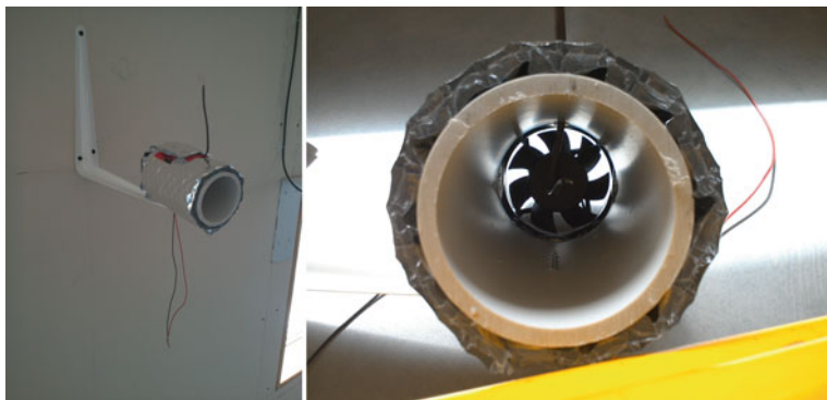
Fig. 7.18 Hand-built air temperature sensing devices used in a lab at Carleton University. The device sucks air through a reflective pipe using a fan to prevent measuring stagnant air or being heated by the sun. The thermocouples are at the centre of the pipe (photo by Sarah Brown, Carleton University)
