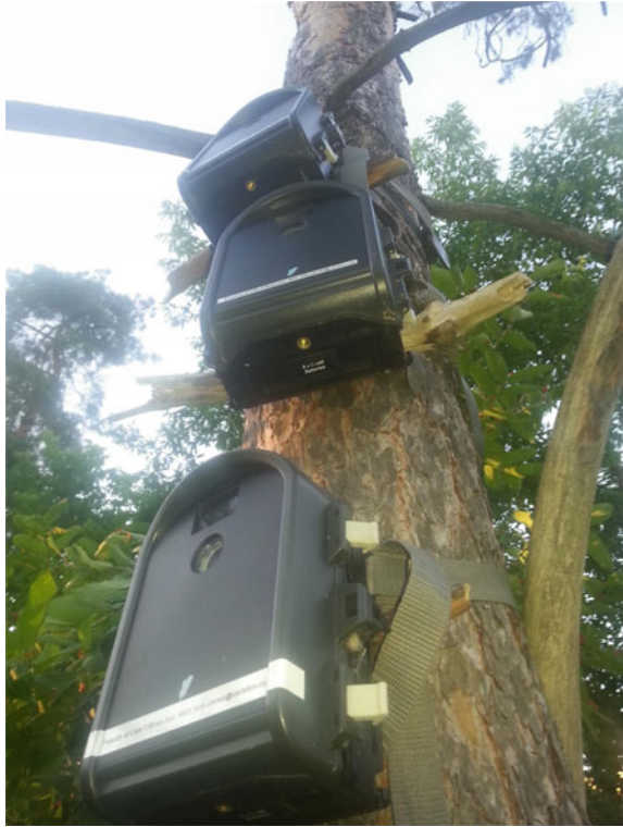
Fig. 6.9 Array of time-lapse cameras, configured to capture an entire façade. Another set of cameras aimed at an oblique angle with respect to the façade was used to detect window opening state
