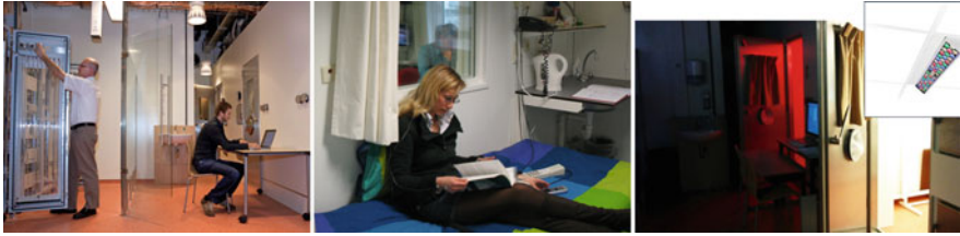
Fig. 7.6 MRUM respiration chambers: overview ( left ), view into one of the chambers with optical connection to the adjacent chamber ( middle ), and light control ( right ) (all photos by MRUM)
