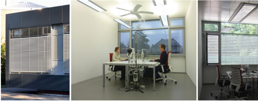
Fig. 7.4 View of the main façade with shadings closed ( left ), interior of the test office spaces with subjects and comfort meter ( middle ) and with shadings closed ( right ) of the LOBSTER at KIT (photos by Moritz M. Karl ( left ) and Marcel Schweiker, KIT)
