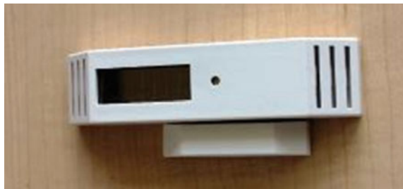
Fig. 6.5 Example of a wireless contact sensor with integrated photovoltaic energy harvesting that communicates with the BAS via a wireless gateway
