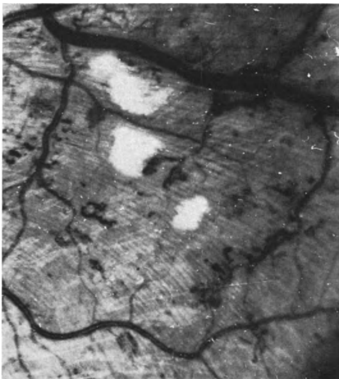
Fig. 14a. Unretouched photograph of a highly enlarged negative, with numerous white spots and lines caused by dust and scratches on the negative (after RIASKOFF, 1972).
