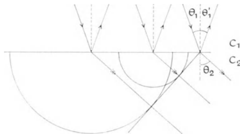
Fig. 5 Construction of the refracted sonic wave front according to the Huygens' principle. \theta_1 equals \theta_1'
