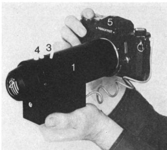
Fig. 10. The E.H.R. photokeratoscope. 1: Extension tube; 2: Target; 3: Diaphragm lever; 4: Flash control; 5: Camera.
