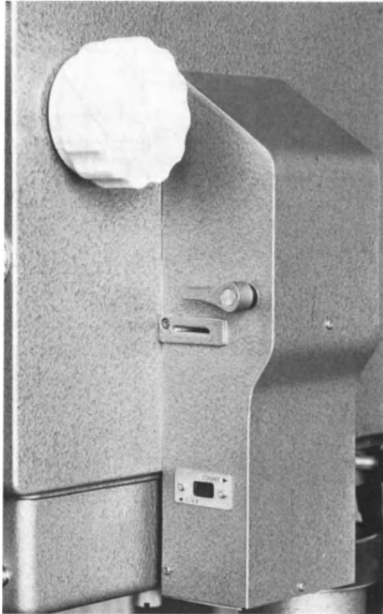
Fig. 11. Digital timer, counter and slot for data plate as used by Topcon.
