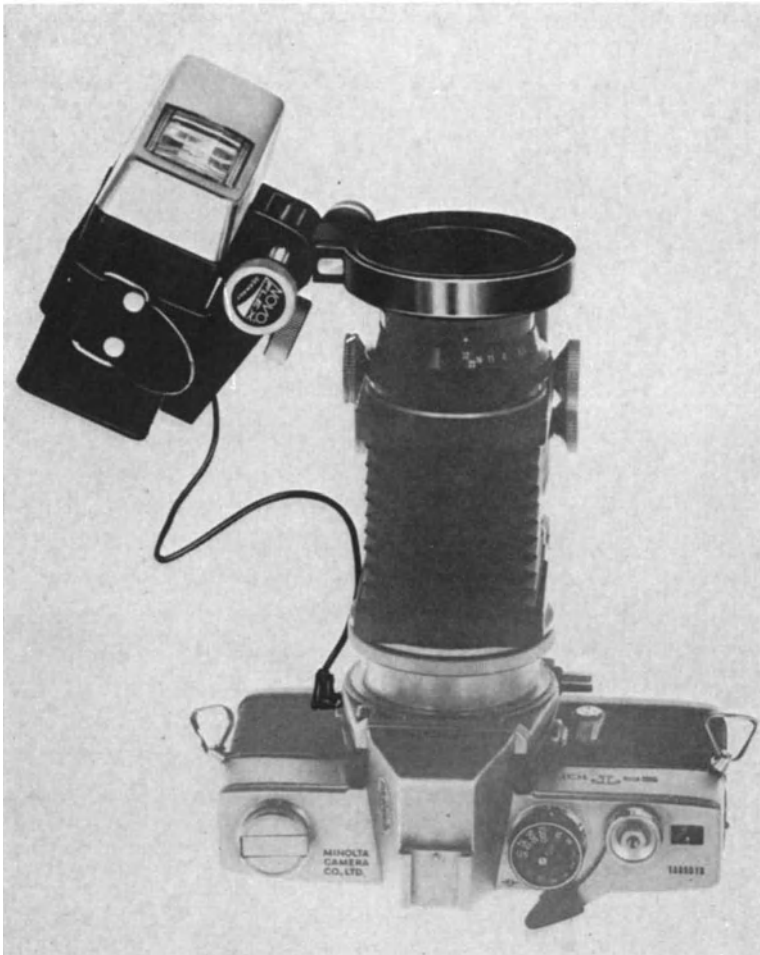
Fig. 2. The ideal set-up for close-up eye photography: 35 mm reflex camera back, automatic extension bellows, 135 mm lens, flash bracket and electronic flash.
