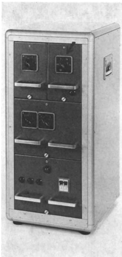
Fig. 6. Power unit of the Zeiss Fundus camera. Arrow: pulse generator.
