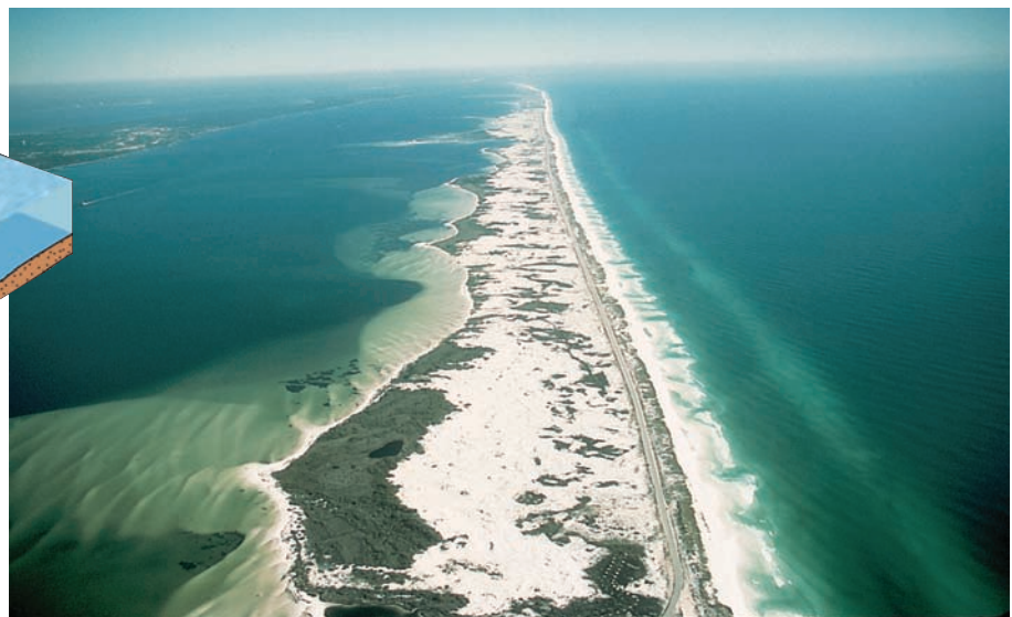
FIGURE 14.18 (A) A barrier island on a gently sloping coast. A lagoon separates the barrier island from the mainland, and tidal currents flowing in and out of gaps in the barrier island deposit sediment as submerged tidal deltas. (B) A barrier island near Pensacola, Florida: open ocean to right, lagoon to left, and mainland Florida on far left. Light-colored lobes of sand within lagoon were eroded from the barrier island by hurricane waves, which washed entirely across the island and into the lagoon. Photo by Frank M. Hanna
