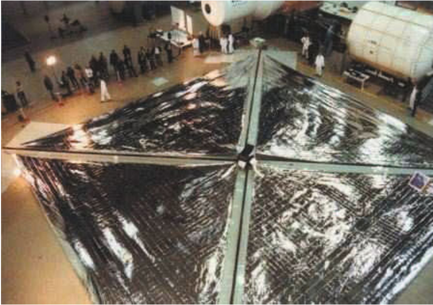
Figure 4. Solar Sails are spacecraft which utilize the momentum transfer of solar photons onto large, highly reflecting sails for passive propulsion. This sail is being developed at the German Aerospace Centre (DLR). Photo credit: DLR.
