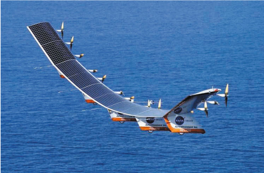
Figure 2. The Helios was designed as a long duration solar powered aircraft. An unexpected, persistent, high dihedral configuration during poor weather on a test flight during June 26, 2003, led to unstable oscillations in a pitch mode and structural failure. Photo credit NASA.
