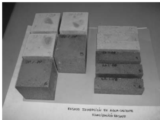
Figure 6. Cubic and prismatic specimens after 17 cycles.
