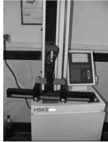
Figure 4. One point flexural strength according to the standard EN12467: 2004.
