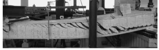
Figure 7. Shear failure of panel P4.
