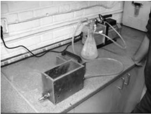
Figure 3. Equipments for preparing the cement boards from cement mortar.
