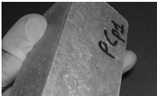
Figure 3. Pathology detail at the end of hot cycle.
