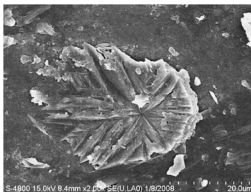
Figure 9. Friedel's salt formation (2000×) on the control specimen in the vicinity of steel/concrete interface.
