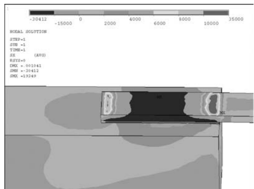
Figure 5. Normal stress distribution after cooling to room temperature.
