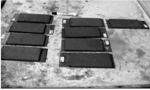
Figure 5. Some samples according to the test EN12467: 2004.
