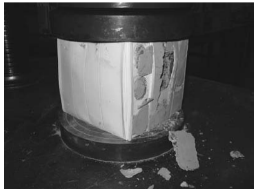
Figure 8. PVC-encased specimen after peak compressive load reached.
