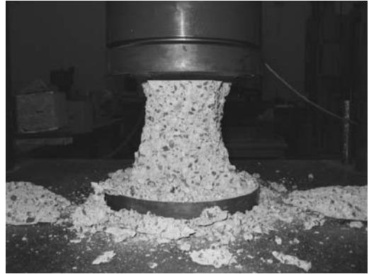
Figure 7. Control specimen after peak compressive load reached.
