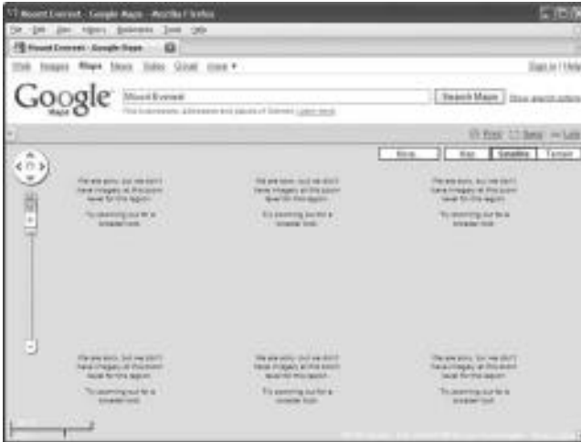
FIGURE 6.15 Tile-based dynamic loading mapping example showing unavailable tiles. (Data from Google Maps.)
