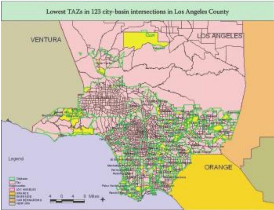
FIGURE 9.10 Identifies the locations of lowest TAZs in the 123 city-basin intersections for storm water treatment plants.
