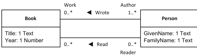
Fig. 8.8 Classes Book and Person interconnected by two associations, and showing roles Work , Author and Reader
