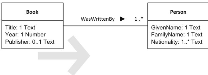
Fig. 8.3 The association in Fig. 8.2, as seen from Book . The large grey arrow, which is not part of the model, can be read as “Every”
