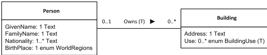
Fig. 15.6 In this diagram, the Building.Use attribute and the Person.Owns semi-association have been marked as temporal
