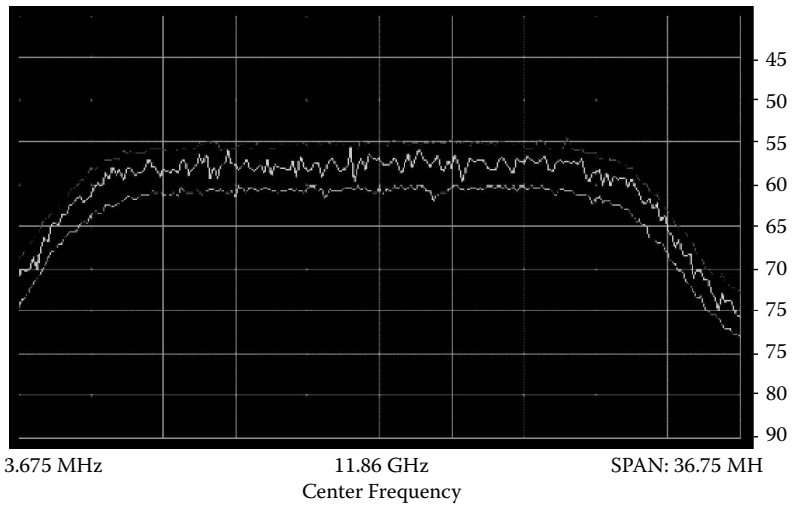
Figure 2.6 Actual plot of signal within a transponder channel.
