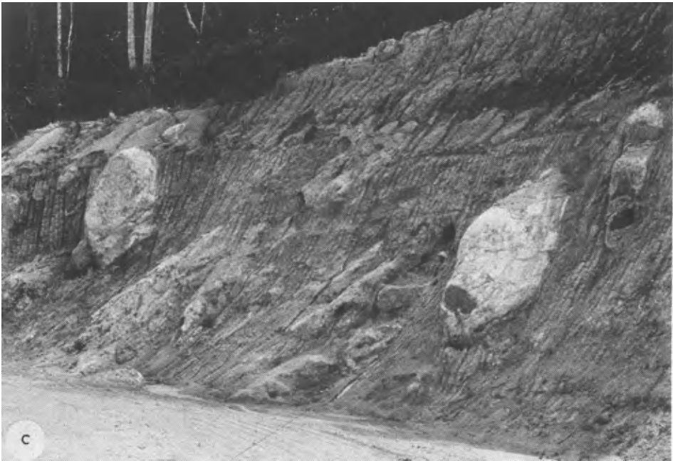
Fig. 4.2 (c). Corestones set in a matrix of grus and exposed near Gemenchah Quarry, West Malaysia, beneath a laterite profile.
