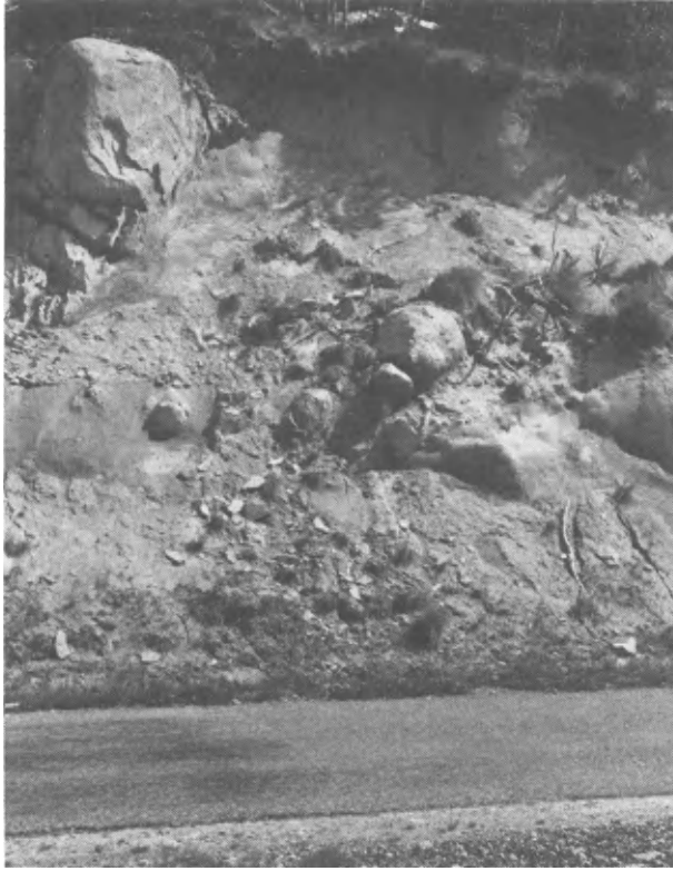
Fig. 4.24. In this 9-10 m deep road cutting in the Snowy Mountains, N.S.W. the grandiorite is deeply weathered, yet a large corestone persists quite close to the land surface.
