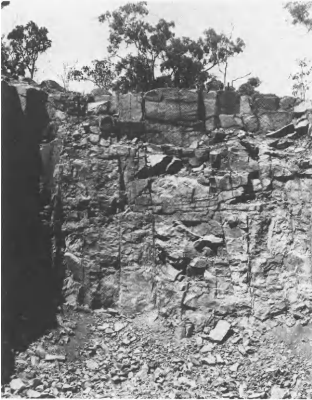
Fig. 2.19. Orthogonal joint sets exposed in quarry at Mt Bunday, near Darwin N.T.
