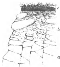
Fig. 4.16. Geikie's (1886) sketch of corestones within a weathered profile: a, solid granite; b, corestones in grus and c, soil.
