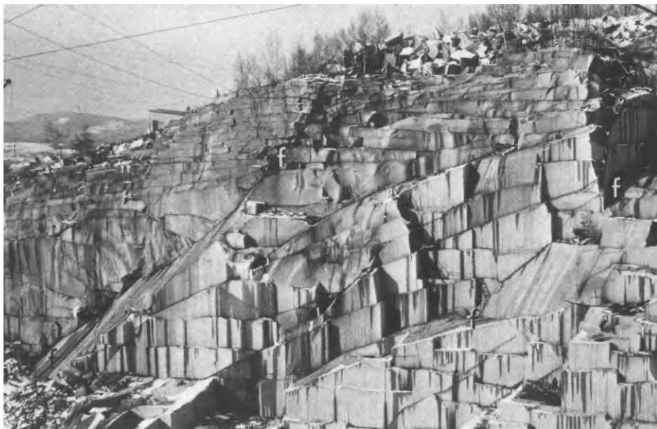
Fig. 2.32. Part of the Rock of Ages Quarry, Barre, Vermont, U.S.A., seen in early 1966, showing sheet structure and fault planes (f) cutting across the sheeting fractures.
