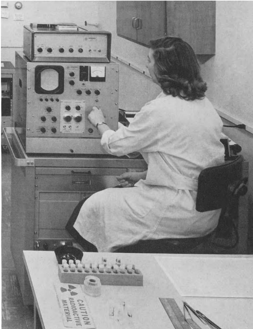
Fig. 6. Photograph of a representative multichannel pulse-height analyzer
