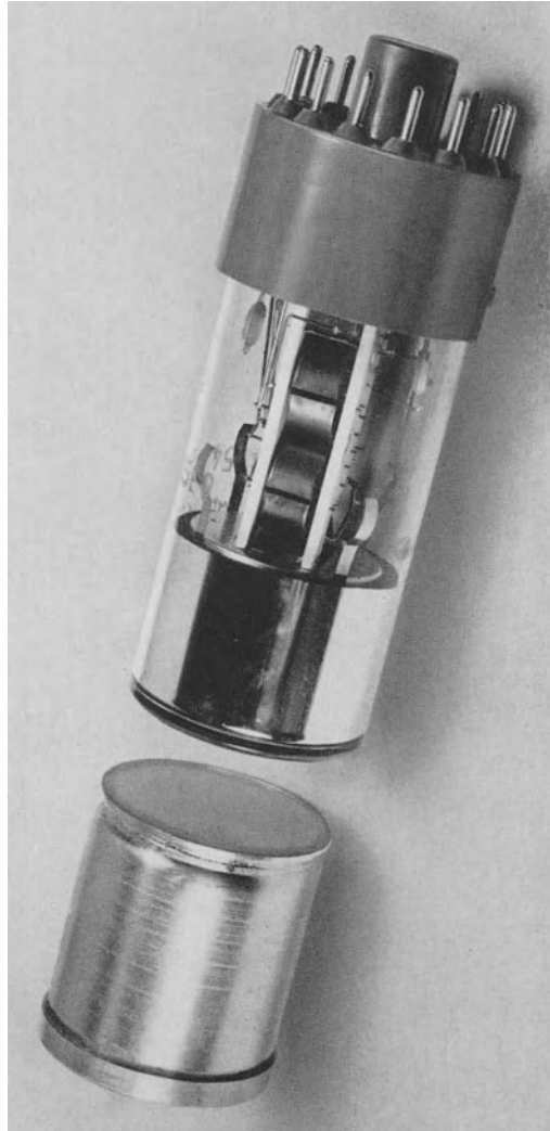
Fig. 4. Exploded view photograph of a NaI(Tl) scintillation counter
