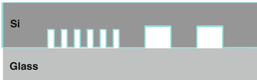
(iv) Anodic bonding of the silicon wafer with a glass wafer
