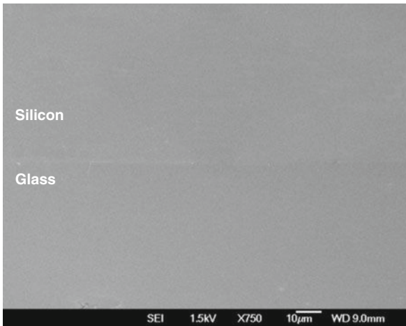
(b) sample D: \text{SiO}_2 + \text{SiN} + \text{SiON}
