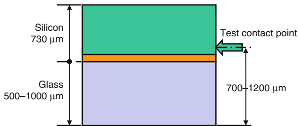
Fig. 9.4 Schematic of the shear test setup. Copyright/used with permission of/courtesy of Institute of Physics and IOP Publishing Limited
