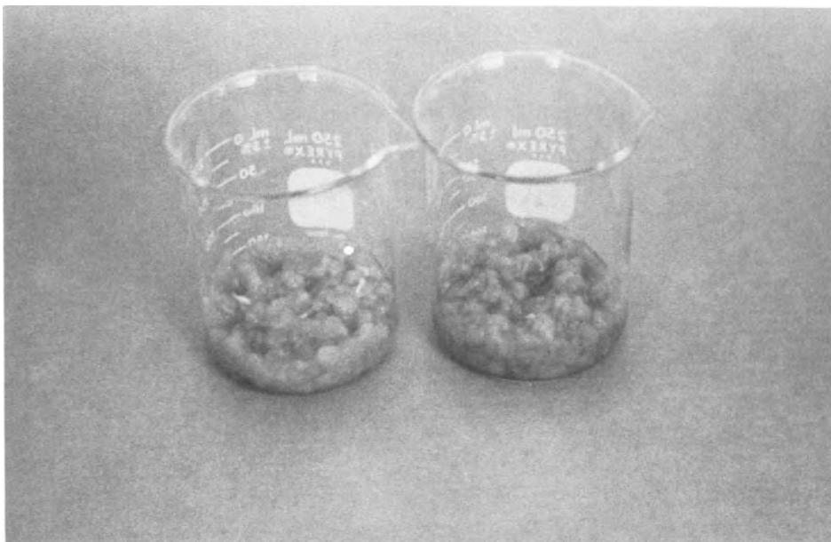
Figure 3. Brightening Effect of Siderophores Isolated from Decay Fungi in Unbleached Pulp Fibers. Siderophore treated pulp (1/2 hour treatment, unwashed) on left. Control unbleached pulp on right.
