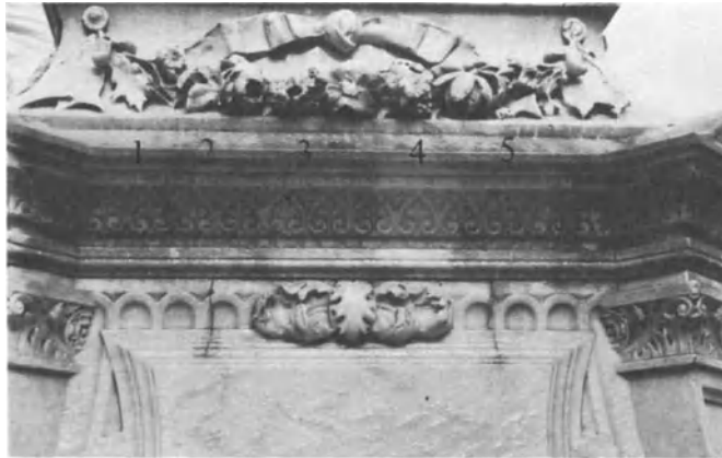
Figure 5. Results of On-Site Tests of Biocidal and Cleaning Treatments. 1) water and detergent, 2) Sure Klean T-1095 Special Liquid Marble Cleaner R by ProSoCo, 3) Sure Klean Marble Poultice and Marble Poultice Additive R by ProSoCo, 4) calcium hypochlorite grains and clay (less than 10% in solution), and 5) 30% hydrogen peroxide solution and clay.
