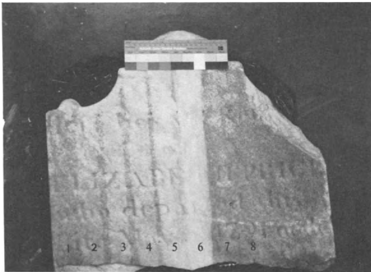
Figure 4. Laboratory Test of Seven Biocidal Cleaning Treatments on a Marble Tombstone Covered with Microorganisms. 1) water and detergent, 2) 30% hydrogen peroxide, 3) 0.75% calcium hypochlorite, 4) 1.5% calcium hypochlorite, 5) 3.0% calcium hypochlorite, 6) calcium hypochlorite grains, 7) Organic Stain Cleanser (Barov, 1987), and 8) a spray of 1% benzalkonium chloride. A clay poultice was used with 2 - 6.
