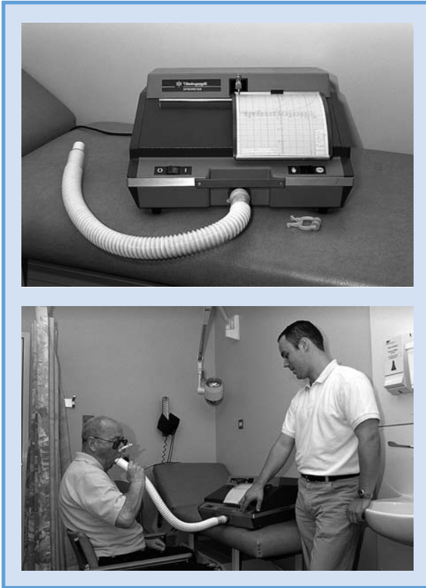
Figure 3.5 A dry-bellows spirometer such as the Vitalograph® is a robust machine suitable for measuring the relationship between volume in time in laboratories and surgery. Other machines based on a pneumotachograph or a turbine measure flow and convert it to volume.
