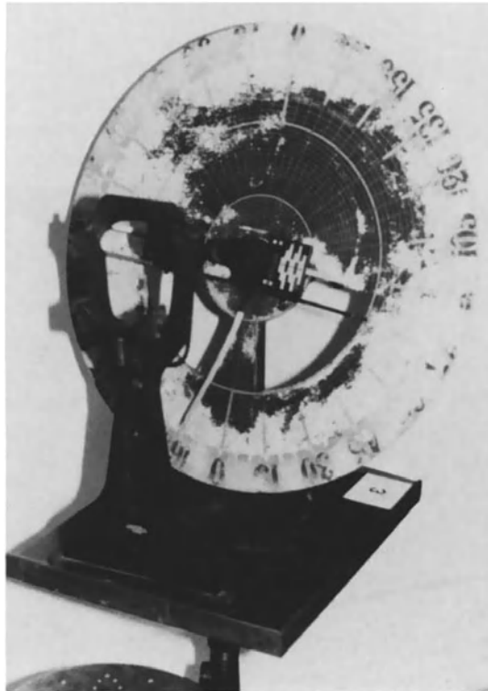
Fig. 8. An early model of Javal's ophthalmometer.
