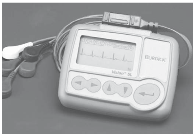
Fig. 13. A version of the Holter monitor that is used currently. The one here is manufactured by Burdick, Inc. (Dearfield, WI).
