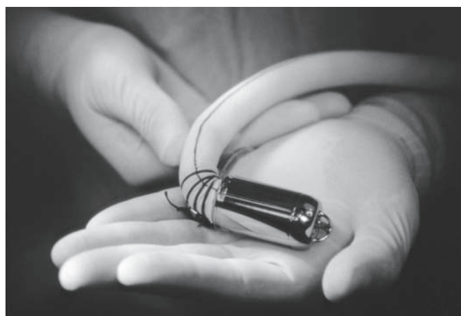
Fig. 4. Size of the Jarvik 2000 (Jarvik Heart, Inc. and Texas Heart Institute) axial flow pump, which like other ventricular assist device systems, has an inlet within the left ventricular apex and outflow connected to the aorta. The advantage of this type of system is that it will likely be totally implantable.
