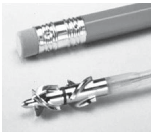
Fig. 3. Relative size of the impeller blade utilized to create flow in the axial pump (compared to a pencil).
