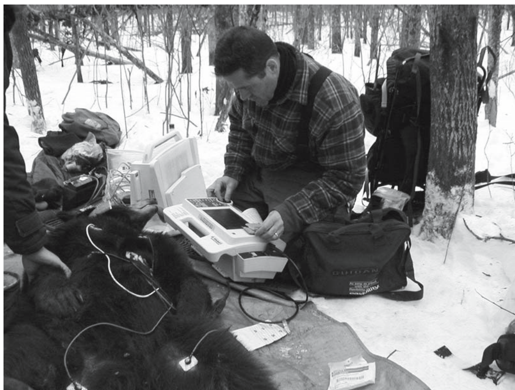
Fig. 3. A LIFEPAK 12 internal defibrillator (Medtronic, Inc., Minneapolis, MN) used externally (outside) on an overwintering black bear. In this case, Dr. Tim Laske is using the system to monitor a 12-lead electrocardiogram (ECG) via its connection to surface electrodes.
