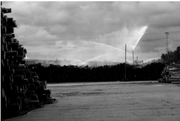
Figure 2.23 Log sprinkling resulting in large amounts of sprinkling water that runs off from a log yard
