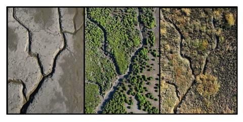
**FIGURE 18.5** Aerial photographs of the same creek network at Pond A21 in April 2008 (2 years post breach), September 2009 (3.5 years post breach), and June 2011 (5 years post breach) illlustrating the rapid sedimentation and natural revegeatation of the marsh. (Photo by Chris Benton.)
