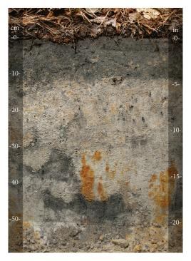
**FIGURE 7.2** Example of iron masses (reddish orange colors) between 30 and 50 cm. (Photo provided by John Kelley.)
