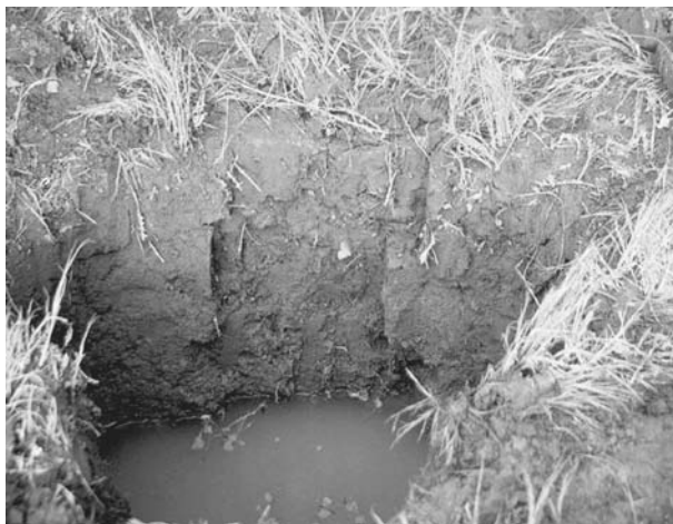
Figure 18.3 Typic Halaquept pedon in a catena affected by seepage from upslope irrigation canals in central Utah. There are no redoximorphic features within 30 cm of the soil surface; the brownish-gray color is inherited from the Mancos Shale parent material. Water level is at 47 cm; pit had to be bailed several times while sampling in November 1996. A Cr horizon occurs at 78 cm. (Photo taken by W.C. Lynn.)
