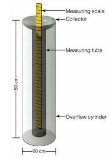
**FIGURE 5.40** Components of the standard rain gauge.
