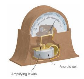
**FIGURE 6.6** The aneroid barometer.
