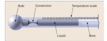
**FIGURE 3.16** A section of a maximum thermometer.
