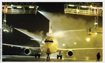
**FIGURE 4** An aircraft undergoing de-icing during inclement winter weather.
