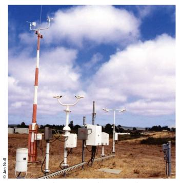
**FIGURE 3.18** The instruments that comprise the ASOS system. The max-min temperature shelter is the middle box.
