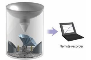
**FIGURE 5.41** The tipping bucket rain gauge. Each time the bucket fills with one-hundredth of an inch of rain, it tips, sending an electric signal to the remote recorder.
