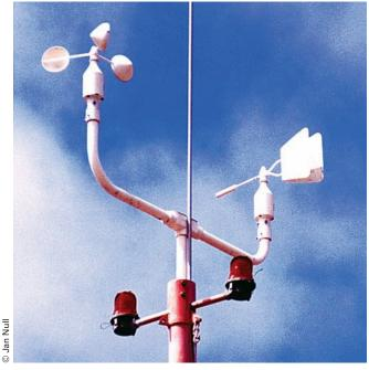
**FIGURE 6.27** A wind vane and a cup anemometer. These instruments are part of the ASOS system. (For a complete picture of the system, see Fig. 3.18, p. 77).
