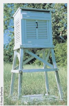
**FIGURE 5** Instrument shelters such as the one shown here serve as a shady place for thermometers. Thermometers inside shelters measure the temperature of the air; whereas thermometers held in direct sunlight do not.
