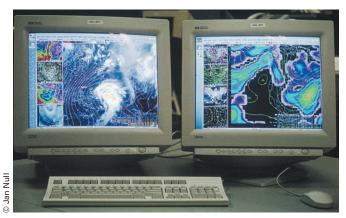
**FIGURE 9.1** The AWIPS computer work station provides various weather maps and overlays on different screens.
