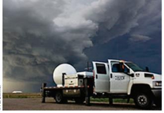
**FIGURE 10.49** Researchers from Texas Tech University set up a mobile Doppler radar unit near a supercell thunderstorm.
