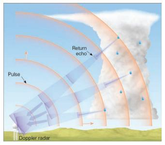
**FIGURE 5.42** A microwave pulse is sent out from the radar transmitter. The pulse strikes raindrops and a fraction of its energy is reflected back to the radar unit, where it is detected and displayed, as shown in Fig. 5.43.
