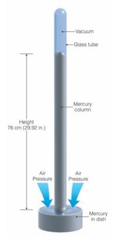
**FIGURE 6.5** The mercury barometer. The height of the mercury column is a measure of atmospheric pressure.
