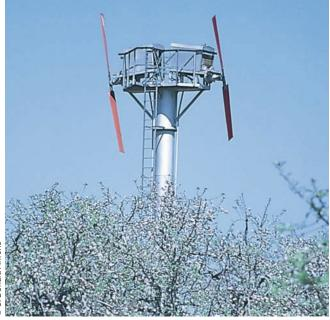
**FIGURE 3.6** Wind machines mix cooler surface air with warmer air above.
