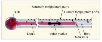
FIGURE 3.17 A section of a minimum thermometer showing both the current air temperature and the minimum temperature in °F.
