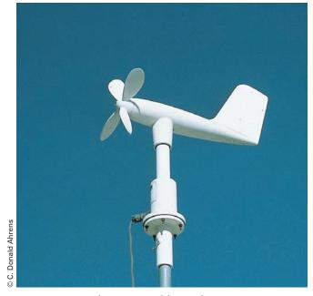
**FIGURE 6.28** The aerovane (skyvane).
