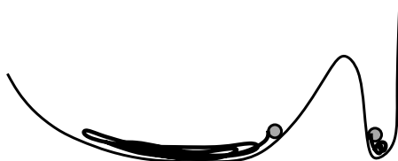
Fig. 3.10. Schematic of a potential and fluctuations. When the slope about the potential minimum is large, the fluctuations are small, and when the slope is small, the fluctuations are large
