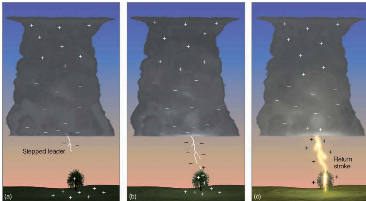
ACTIVE FIGURE 14.31 The development of a lightning stroke. (a) When the negative charge near the bottom of the cloud becomes large enough to overcome the air's resistance, a flow of electrons—the stepped leader—rushes toward the earth. (b) As the electrons approach the ground, a region of positive charge moves up into the air through any conducting object, such as trees, buildings, and even humans. (c) When the downward flow of electrons meets the upward surge of positive charge, a strong electric current—a bright return stroke—carries positive charge upward into the cloud. Visit the Meteorology Resource Center to view this and other active figures at academic.cengage.com/login
