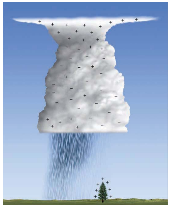
● FIGURE 14.30 The generalized charge distribution in a mature thunderstorm.
