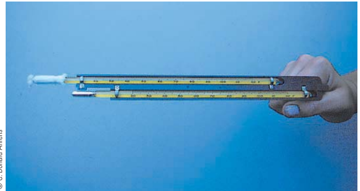
● FIGURE 4.20 The sling psychrometer.
