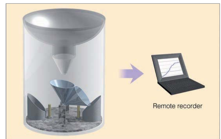
● FIGURE 7.32 The tipping bucket rain gauge. Each time the bucket fills with one-hundredth of an inch of rain, it tips, sending an electric signal to the remote recorder.
