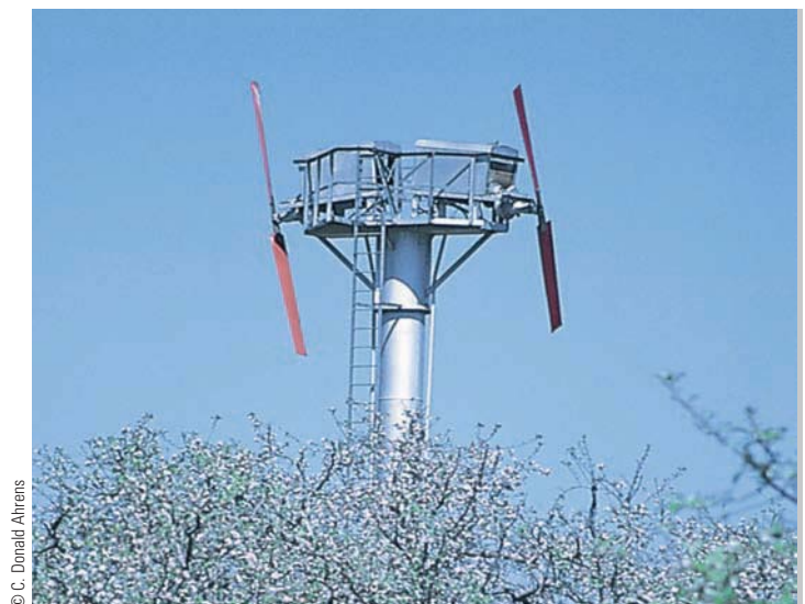
● FIGURE 3.19 Wind machines mix cooler surface air with warmer air above.
