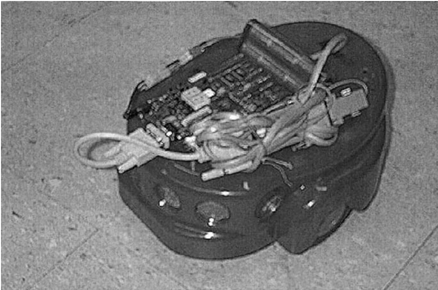
Figure 13.27 ActiveMedia's Amigobot robot base controlled by an FPGA with a Nios Processor
