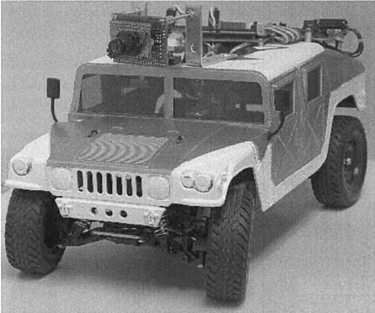
Figure 13.25 Hobbyist R/C model with a CMU camera and R/C PWM servos controlled by an FPGA
