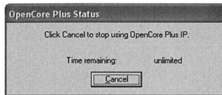
Figure 16.9 Keep this dialog box open as long as the FPGA is being used.
