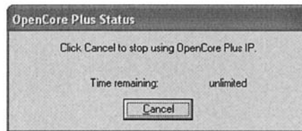
Figure 16.22 Keep this dialog box open as long as the FPGA is being used.
