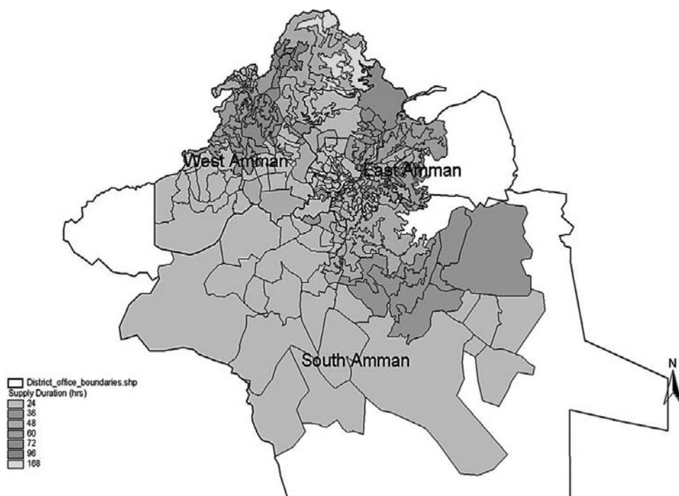
Figure 28.4. The total supply duration (hours per week) in Greater Amman, summer 2006. Source: LEMA Company, personal communication, Amman 2007. See colour plate section.
