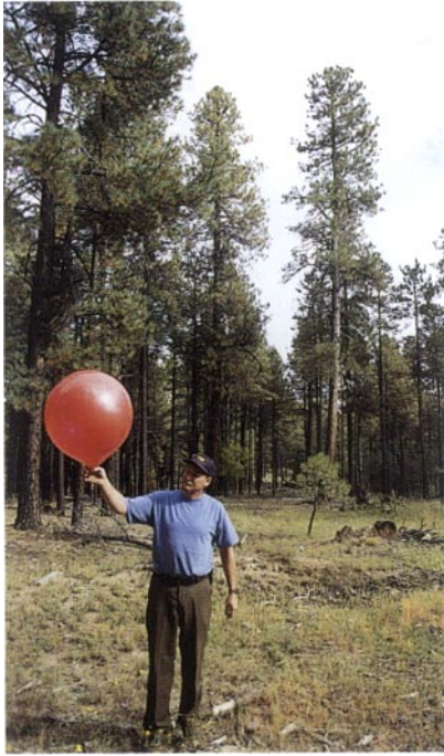
Figure 13.23 Releasing a pilot balloon to determine the speed and direction of winds that affect a fire. (Photo © A. Farnsworth)
