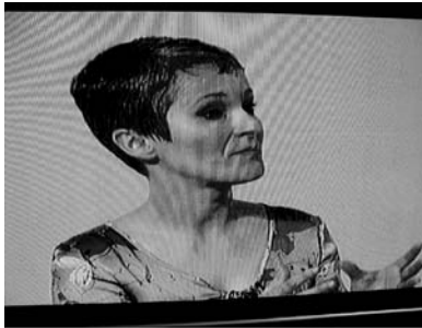
(c) LVDS connector dislodged slightly – one data pair disconnected
