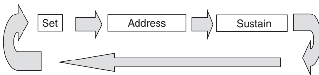
Figure 10.7 Three-phase pixel cell drive cycle
