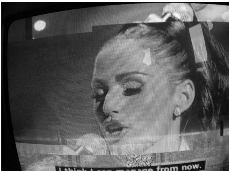
Figure 18.27 Symptoms of a partial fault of video memory (address line stuck at zero showing image blocks in wrong places)
