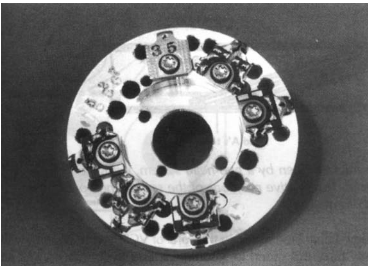
Figure 21.14 Video head drum. This photograph of the underside shows five heads with a 'blank' (for mechanical balance) near the top. The heads at one o'clock and seven o'clock are double types for video, the others for hi-fi audio (two o'clock and eight o'clock) and flying erase near the bottom
