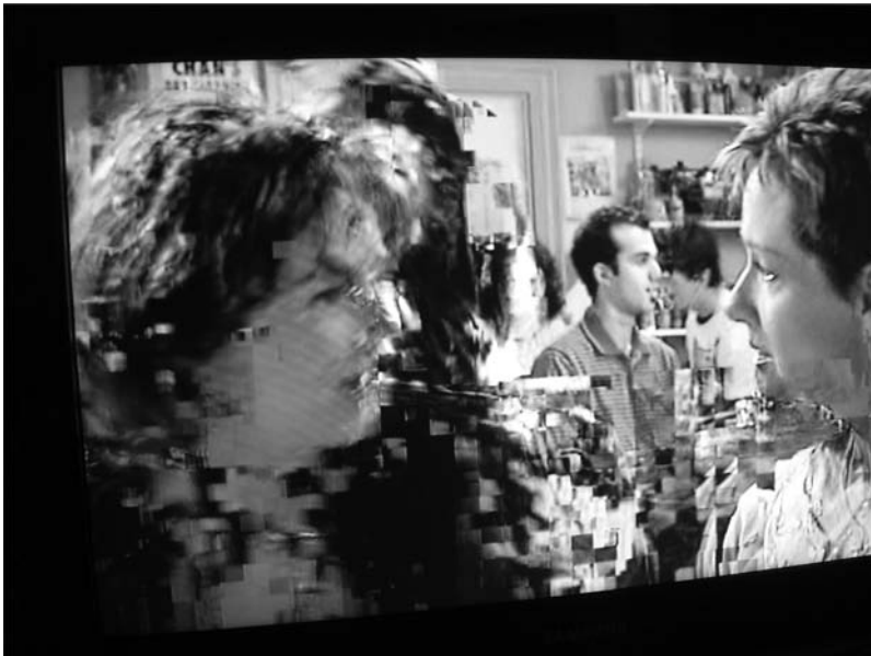
Figure 18.23 Pixelisation due to high BER count
