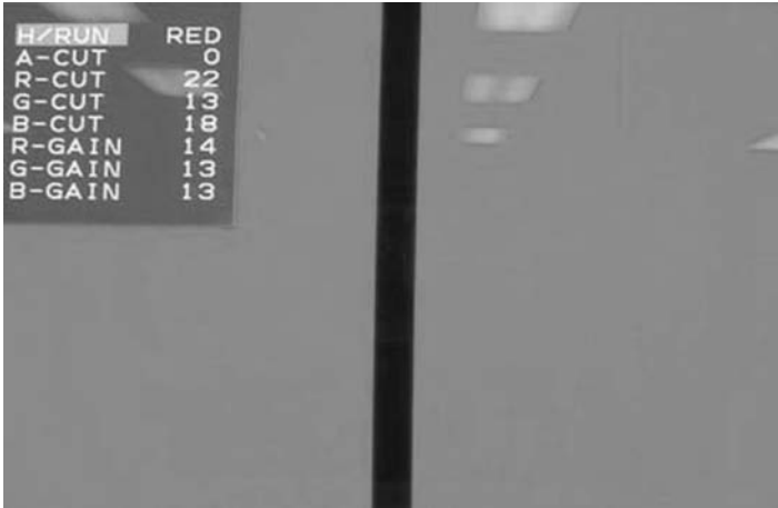
Figure 11.33 Source or column drive fault
