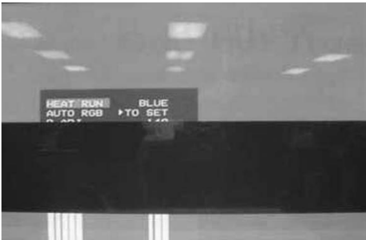
Figure 11.34 Symptom of a line gate driver fault
