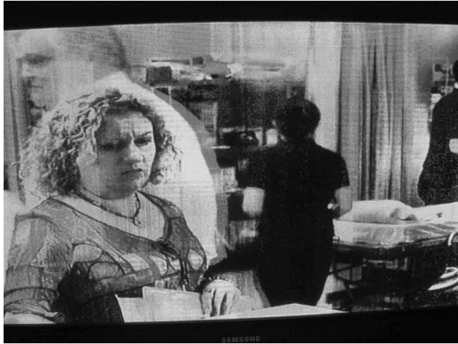
Figure 10.26 Effect of maladjusted ramp set pulse
