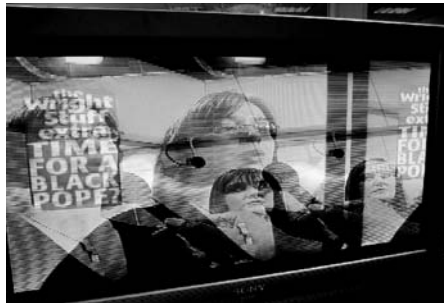
(e) Scan Memory fault (address line shorted to 0V)
