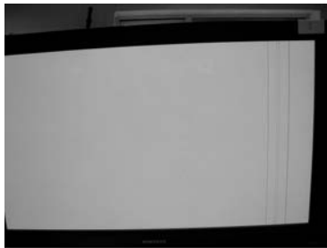
C Multiple vertical lines – faulty Tape carrier
